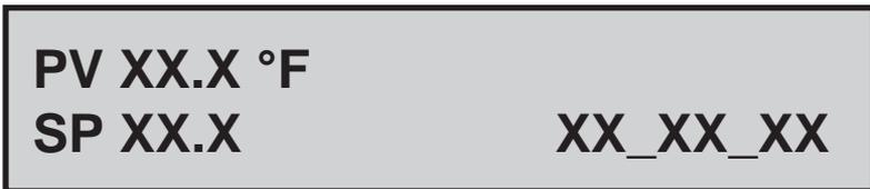
FIGURE 33. DISPLAY OF PROCESS VARIABLES/SETPOINT IN RUN MODE - ON
