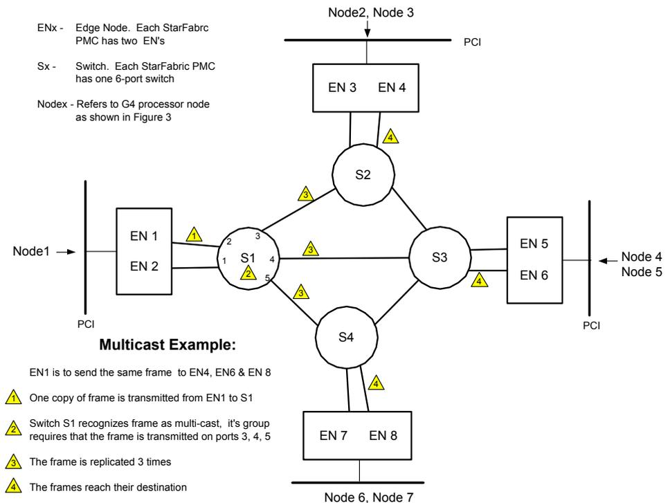
Figure 5: Multicast Example
