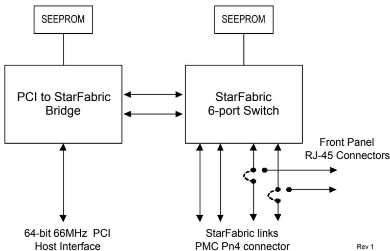
Figure 1: StarLink Block Diagram
