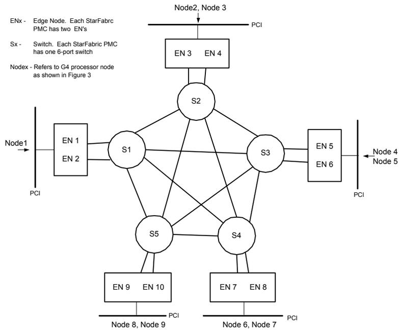
Figure 2: Application Example: Network Topology
