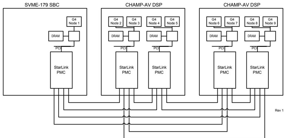
Figure 3: Application Example: System Block Diagram
