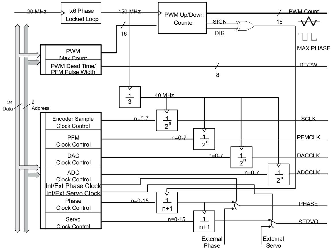
Figure 3 PMAC2 Gate Array IC Clock Control
