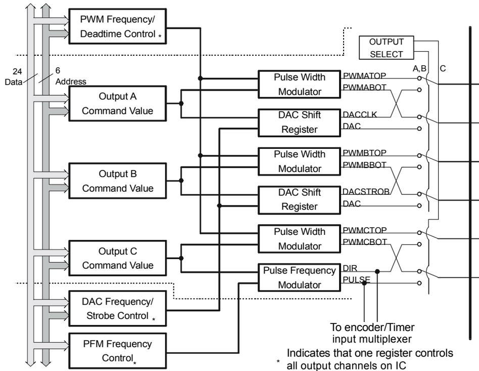
Figure 4 PMAC2 Gate Array IC Output Channel
