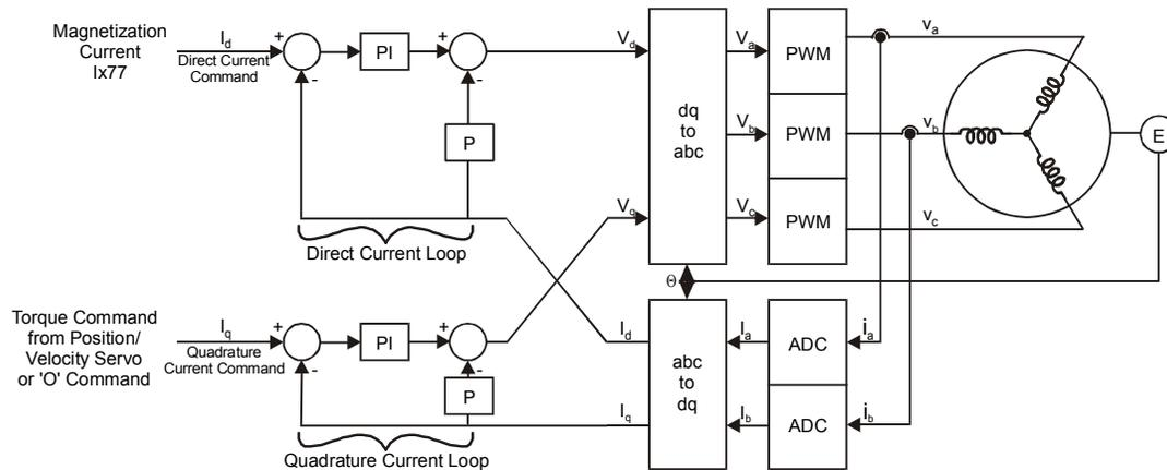
Figure 9 PMAC2 Commutation with Digital Current Loop
