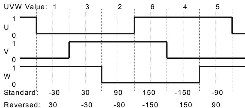
**Figure 13 Hall-Effect Waveforms With Zero Offset**
