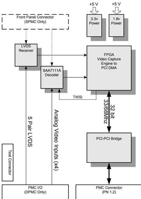
Figure 1: PMC-724 Frame Grabber Block Diagram
