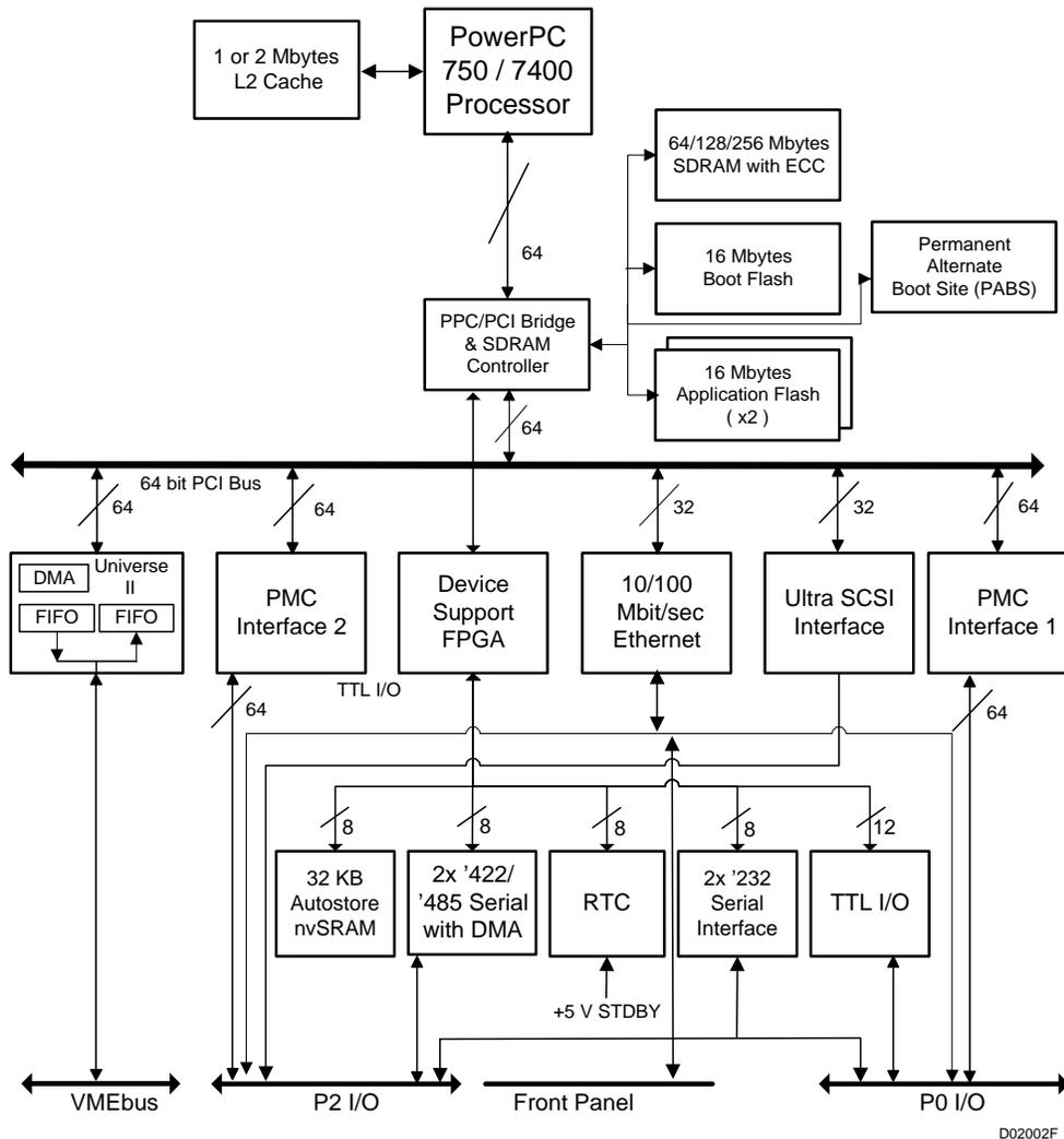
Figure 1: Block Diagram (see Table 3 for alternate I/O Routing)
