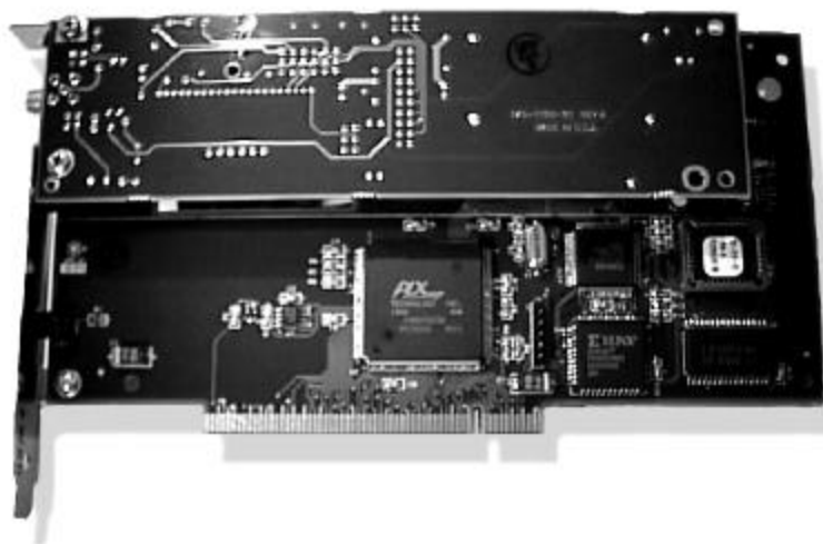
Figure 4.3 PCLTA-20 SMX Interface and PCLTA-20 Protocol Analyzer with PLM-22 SMX Transceiver Installed
