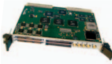
Echotek's dual-channel programmable A/D converter samples data at 1.5 GHz for high-speed, signal-processing tasks.
