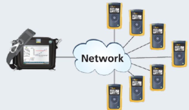
Test from one location with the MetroScope to multiple LinkReflectors in the field
