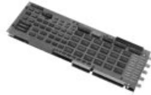
DSPLINK is a 32 bit mezzanine bus supported by Digital Signal Processing cards from a number of vendors. It allows data to be transferred from the data buffer on a CompuScope 1012 card to a DSP card without having to go through the ISA bus.
