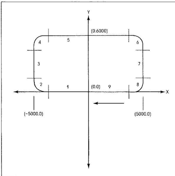
Figure 3. Scribing a Rectangle with Radiused Corners
