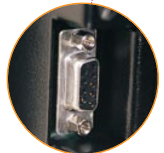
Communications Port RS-232 port for easy PC and modem connections
