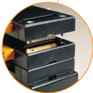
Modular Construction SmartStack modular I/O stacks up to four deep
