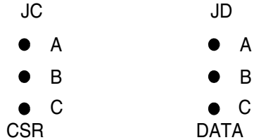
c. AM2 Jumpered for Short Supervisory Access (no jumpers installed)
