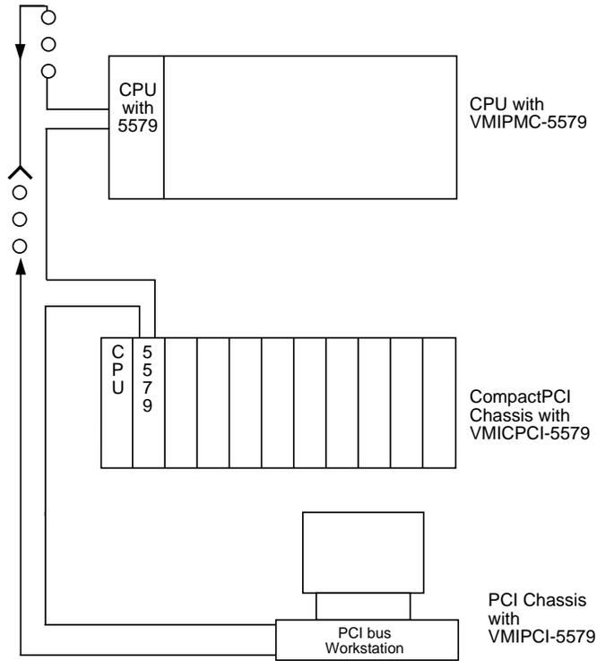
**Figure 1. Network Example Using Reflective Memory System**
