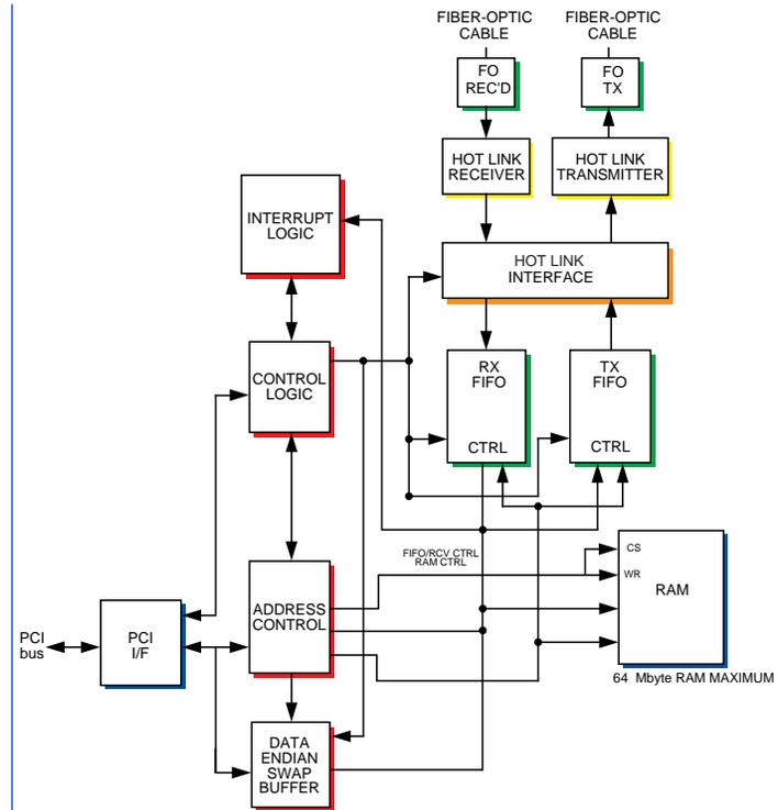
**Figure 2. VMIPMC-5579 Functional Block Diagram**
