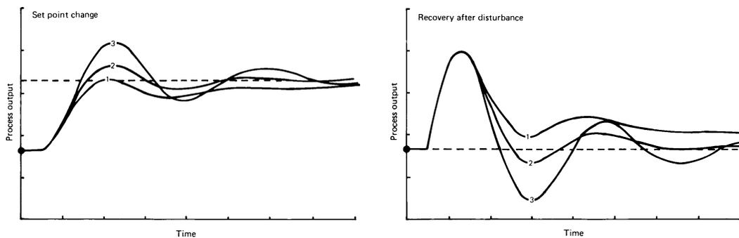
FIGURE 2-2 Integral Gain Effects on Response
