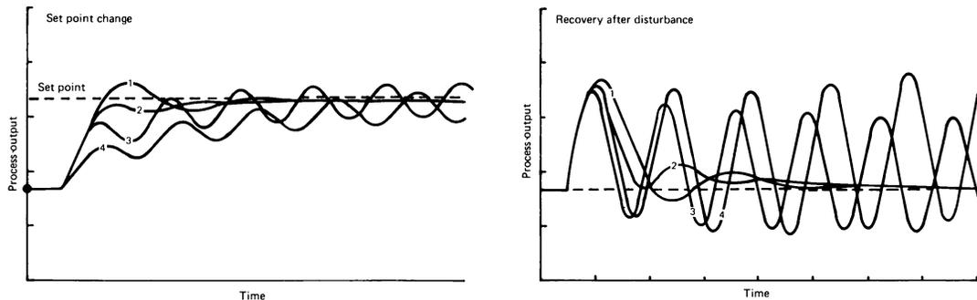
FIGURE 2-3 Derivative Gain Effect on Response
