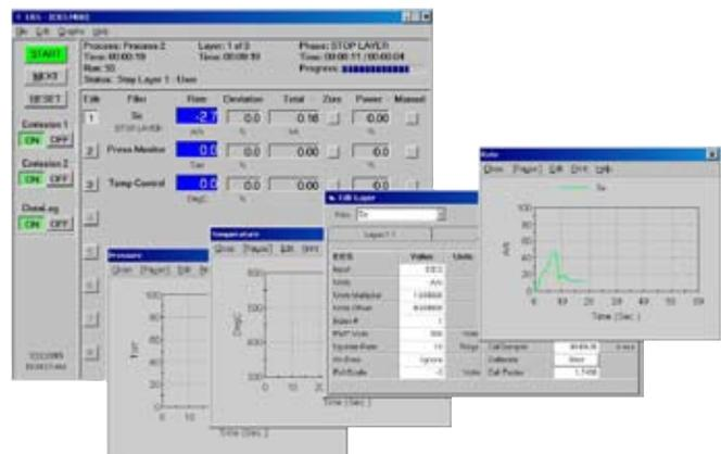
Figure 2 - Guardian software provides all of the functions required for an eight sensor, eight output, multi-layer co-deposition controller. Process settings, numeric data, and graphs can be displayed during all phases of deposition.
