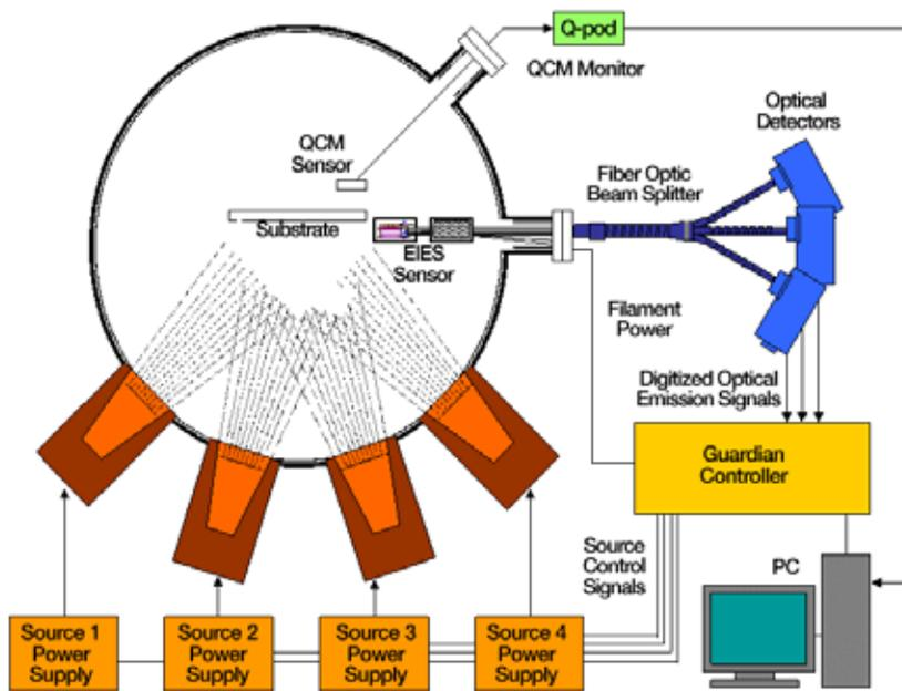
Figure 1 - Typical system configuration.
