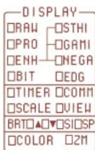
**ENH Enhance:** Allows interactive enhancement, suppression, or isolation of selected intensity levels on the image. Fourteen different enhancement modes are available, of which any three can be selected for display on the main menu.
