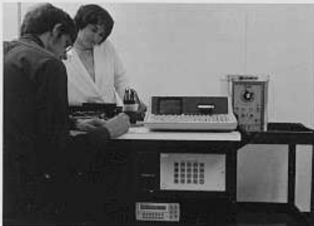
Production testing of temperature probes.
