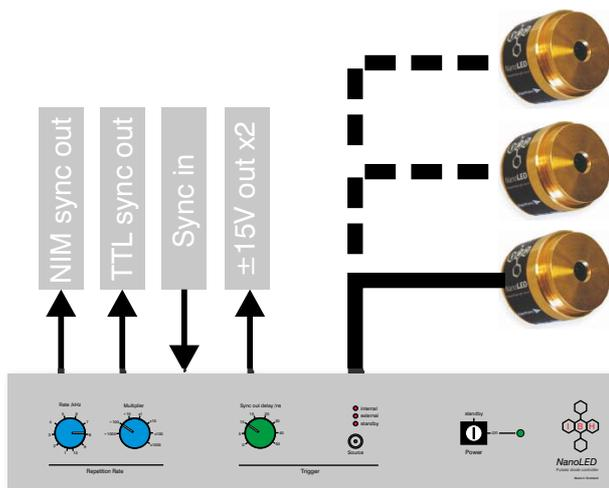
All NanoLED sources (LED and laser) operate in conjunction with the Controller - a rack-mountable module containing power supplies, master oscillator, and synchronisation circuitry. The fast drive electronics are contained inside the sources, allowing each to be optimised independently of the Controller. This ensures that sources can be interchanged, quite literally, in seconds.
