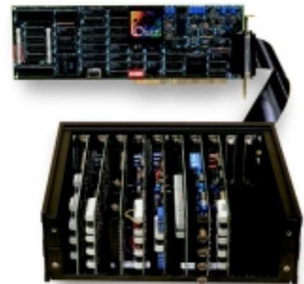
For large systems, the DBK41™ ten-slot expansion module attaches to the DaqBoard P1 analog I/O connector to accommodate any combination of analog DBK signal conditioning and expansion cards. The cards simply plug into the backplane of the DBK41; the unit, which is shown with the cover removed, accommodates up to 10 analog cards. A CA-131-1T ribbon cable attaches the DBK41 module to the DaqBoard P1 analog I/O connector.
