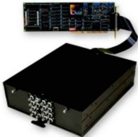
The DaqBoard attaches easily to the DBK60™ expansion module which provides three slots for signal conditioning cards and a choice of termination panels.
