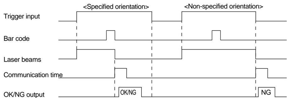
An reading error is issued when the unit reads a bar code label running in the orientation which is not specified.
