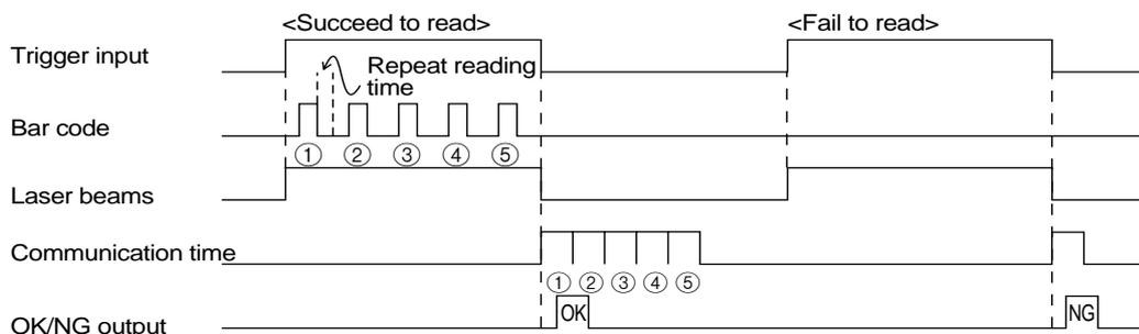
Multi 2 mode allows the unit to read several bar codes while the trigger input is on (or during the preset input time if one-shot signal trigger is selected) and sends all the readout data at one time after the trigger input turns off (or after the preset input time is expired if one-shot signal trigger is selected).
