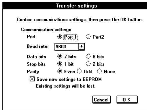
2. Set the baud rate, data bits, stop bit and parity according the BL-500's settings. The BL-500's default settings are shown above.
