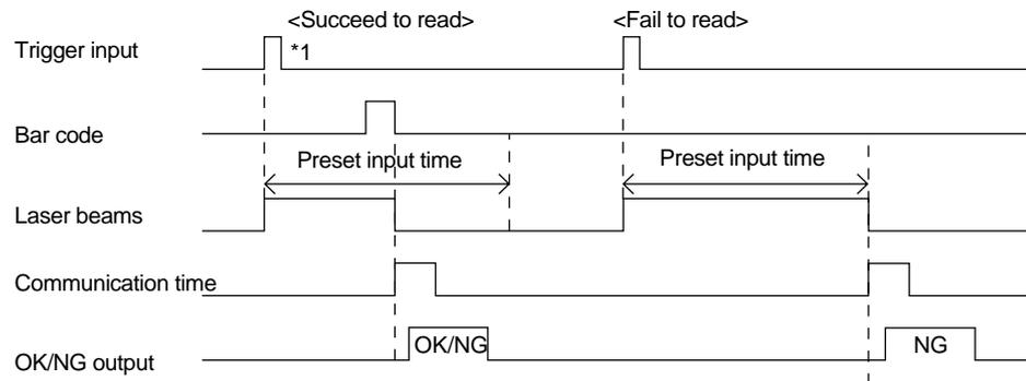
1. After the trigger input exceeds the preset input times, the laser begins to emit.
