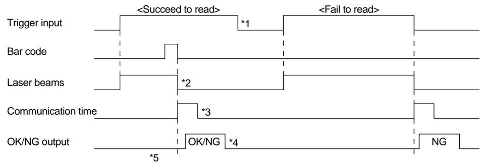
1. Set trigger input so that it stays on long enough for the laser beam to cover the entire bar code.
