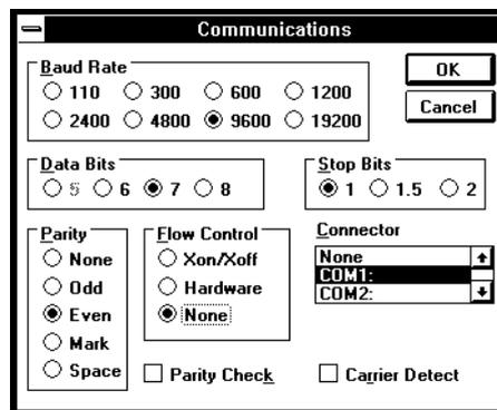
After setting “Connector” to COM1 or COM2, set the baud rate, data bits, stop bits and parity according to the BL-500’s settings. When the data bits is set to “8 bits”, the parity can only be set to “None.”
