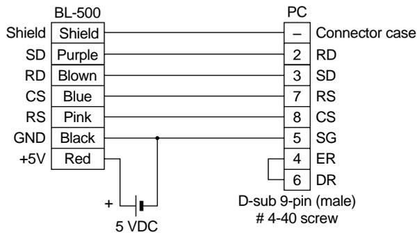
Use a metallic connector housing for the D-sub 9-pin connector. Connect the shielded cable with the connector housing.
