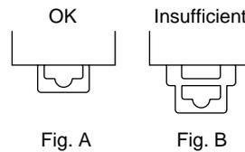
3. To remove the BL-U1 from the DIN rail, pull out the notch until its shape turns from Fig. B to Fig. A. Then, disengage the BL-U1 from the DIN rail.
