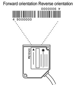
Normally, the unit can read bar codes regardless of the orientation.
