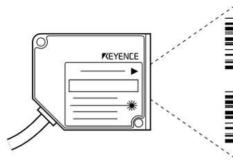
If you use multi-label read mode (multi 3), the BL-500 can simultaneously read 2 to 4 bar codes in the field of the laser beam.
