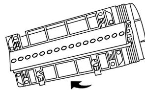
2. Check that the DIN rail mounting notch is shaped like notch A below. If not, push the BL-U1 further.
