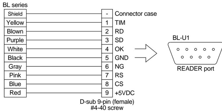
Use a metallic connector case for the D-sub 9-pin connector and connect the shielded line to the connector case. This allows connection to the earth ground of the AC power cable.
