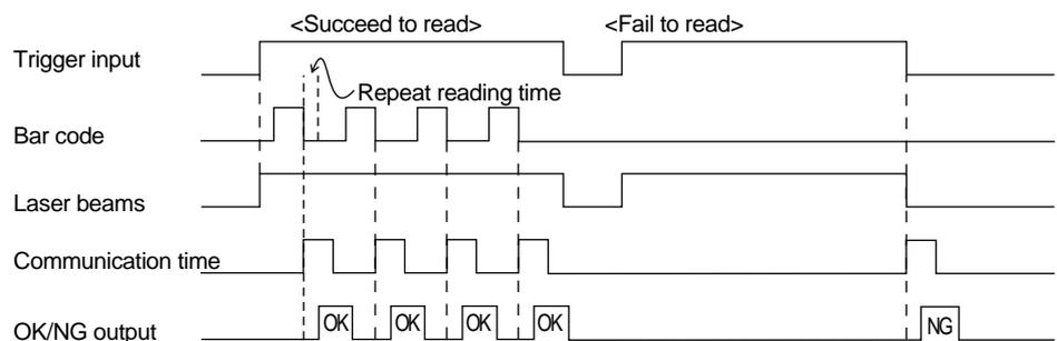
In the multi-label read mode 1, the unit reads several bar codes continuously, and outputs them sequentially as it reads while laser beam remains on and trigger input turns on after bar codes have been read (or during the preset input time if one-shot signal trigger is selected).
