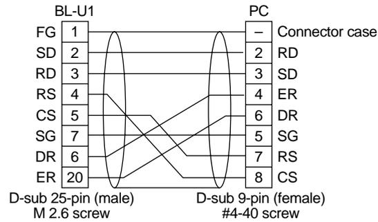
Be sure to use a metal connector case for the 9-pin D-sub connector. Connect the connector case to the shield wire.
