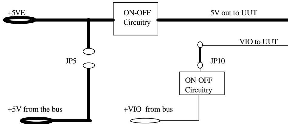
As indicated, there will be conflict in case the external supply is connected while the jumper is still in place. This circuit is repeated for each of the 4 voltages.
