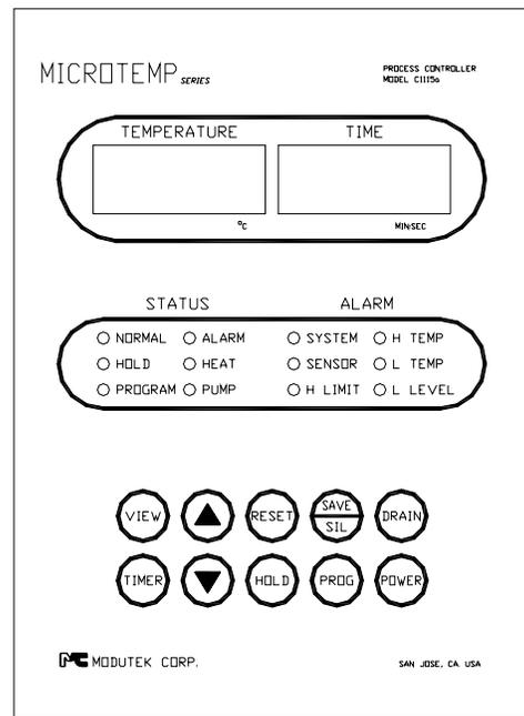
Figure 3.1a, b,c,d - MICROTEMP PCT Front Panel
