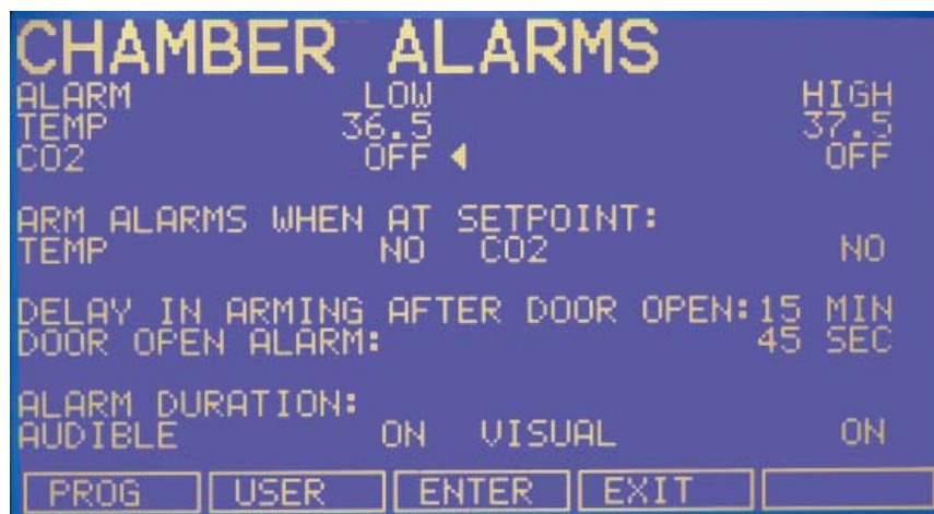
Figure 11: CHAMBER ALARMS Programming Screen
