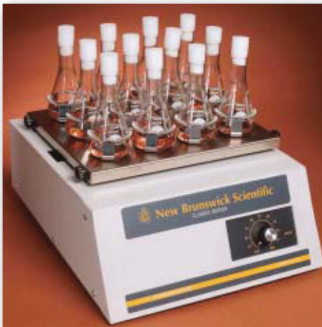
Model C1 Gyrotary Shaker with dedicated platform for 12 size 125 ml flasks.
