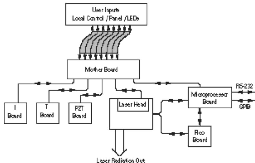
The analog layer consists of four printed circuit boards: the current board, the temperature board, the piezoelectric-transducer (PZT) driver board which controls wavelength fine tuning, and the Picomotor control board for coarse wavelength tuning. The digital layer includes the microprocessor board and the mother board. There is another digital circuit board in the laser head that
