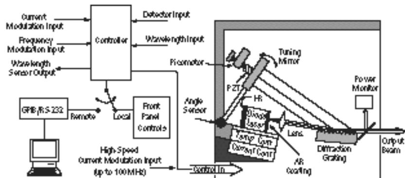
In this design, a diode laser is used as the gain medium. One end of the diode laser has a high reflectivity coating which acts as an end mirror of the external-cavity. The other end of the diode has an antireflection coating.
