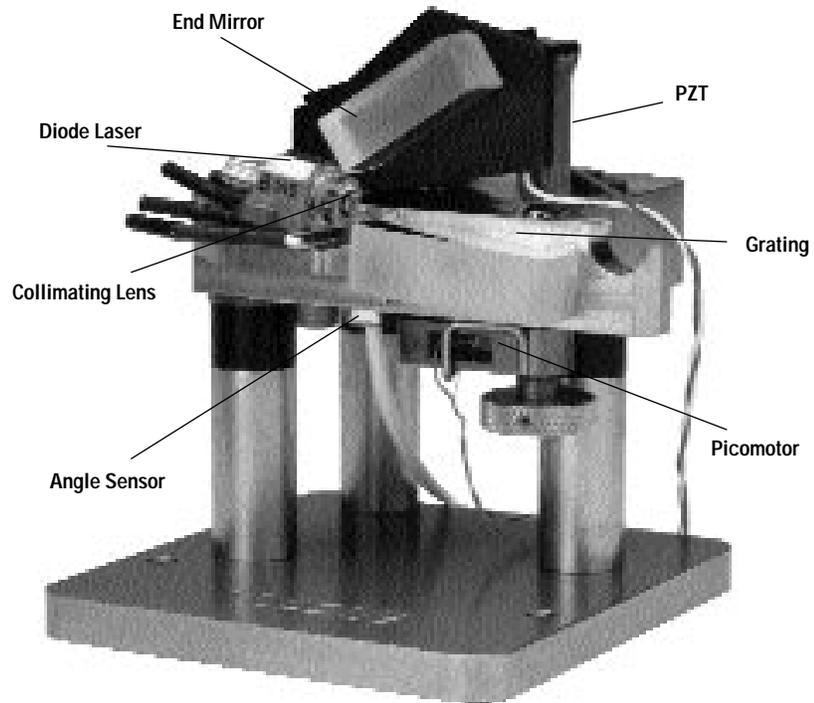
from the diode is reflected, not diffracted, by the grating. This portion forms the output beam.
