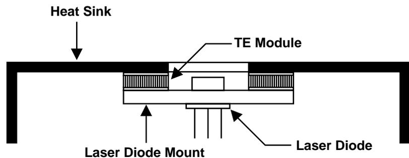
Figure 4: Mounting arrangement of a TE module, heat sink and laser diode
