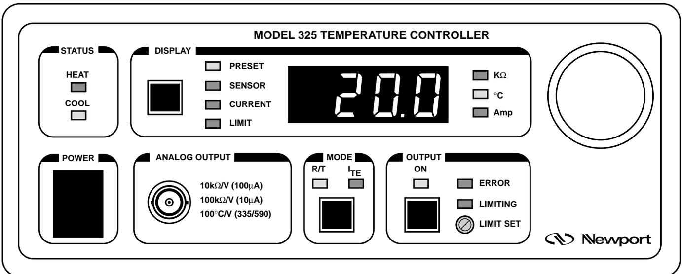
Figure 1: Front panel layout
