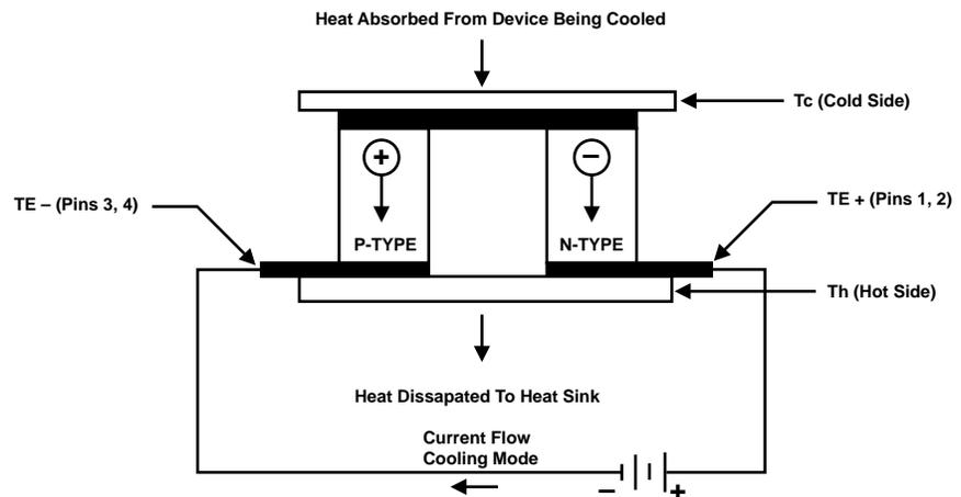
*Figure 3: TE module configuration*
