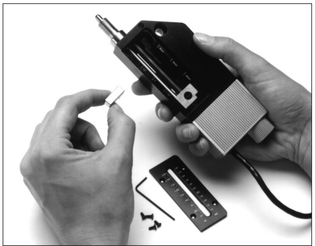
Figure 4 - Place the half nut on the leadscrew to set the approximate travel.
