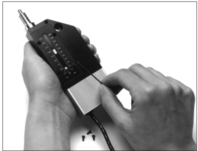
Figure 6 - Tighten all four screws securely for proper operation.
