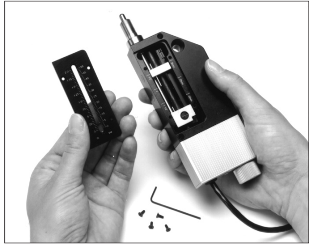
Figure 2 - Approximate travel range markings assist in quick travel adjustment.
