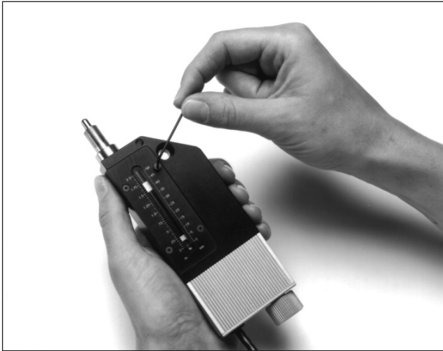
Figure 1 - Remove the indicator window lid with the actuator in the zero position.
