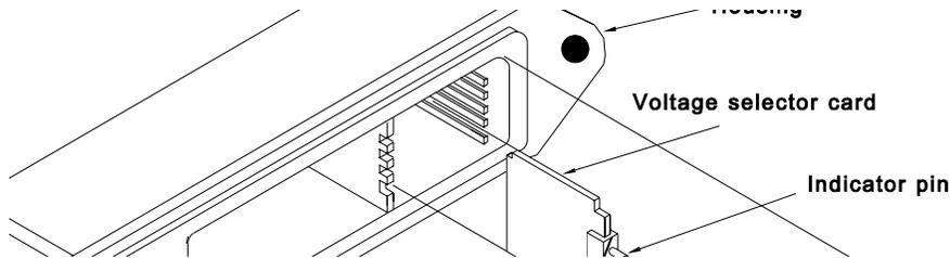
**Figure 1 Power Input Connector**
