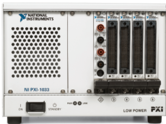
Figure 1. Expand channel count with PXI switching.
