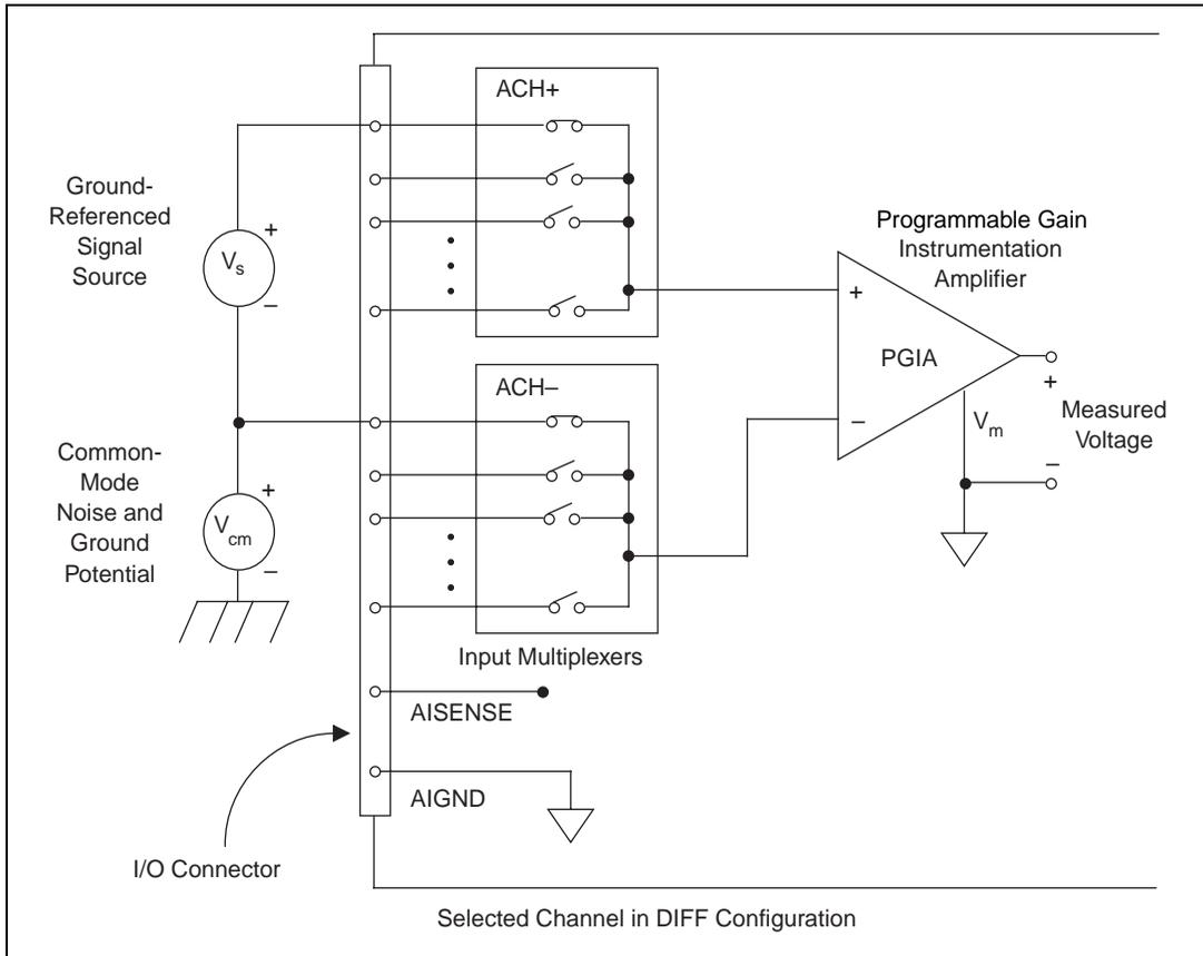
**Figure 4-4.** Differential Input Connections for Ground-Referenced Signals
