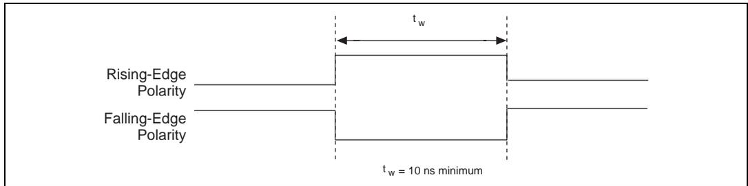
**Figure 4-30.** GPCTR0\_GATE Signal Timing in Edge-Detection Mode
