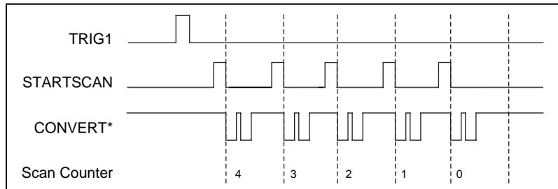
Figure 4-11. Typical Posttriggered Acquisition
