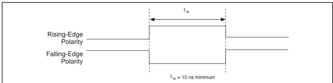
**Figure 4-33.** GPCTR1\_GATE Signal Timing in Edge-Detection Mode
