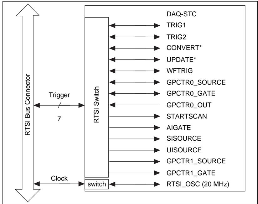
**Figure 3-3.** PCI RTSI Bus Signal Connection
