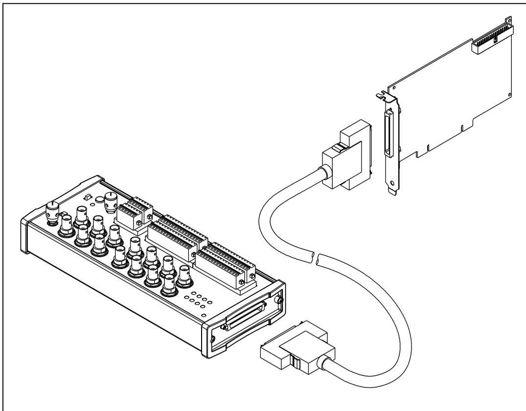
**Figure 1.** Connecting a BNC-2121 to a 660X Device
