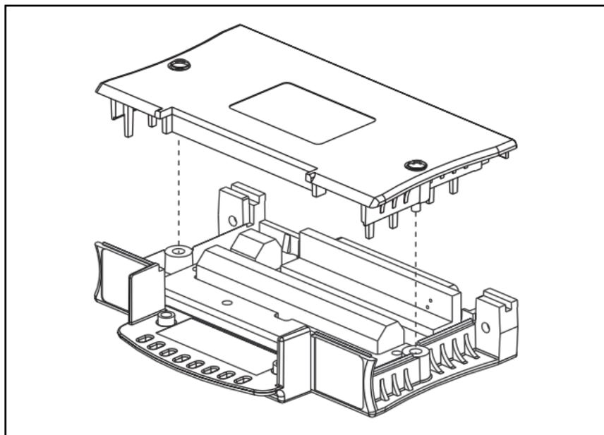
**Figure 3.** Removing the Top Cover from the cFP-CB-*x*
