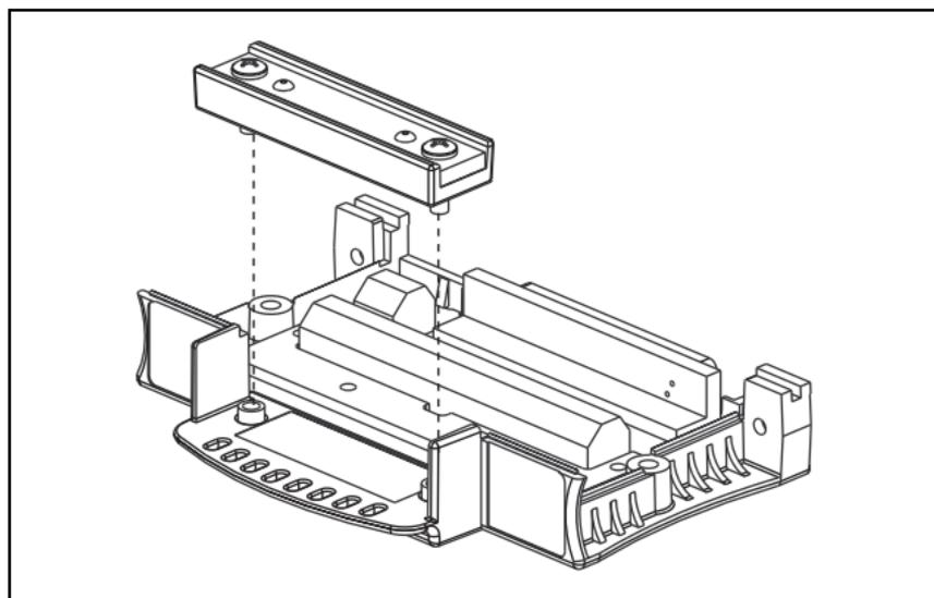
**Figure 5.** Installing the Strain-Relief Bar
