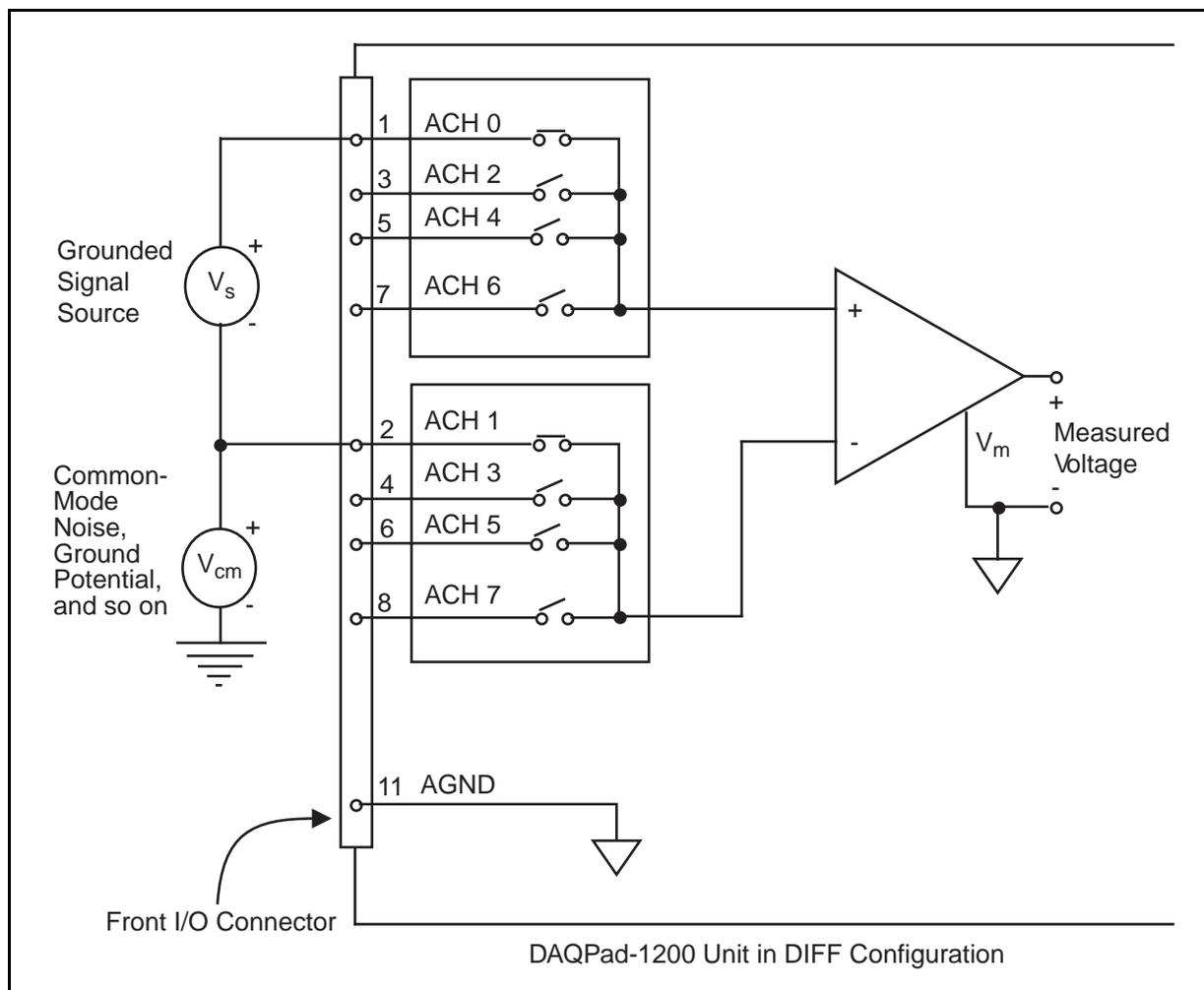
Figure 3-4. Differential Input Connections for Grounded Signal Sources
