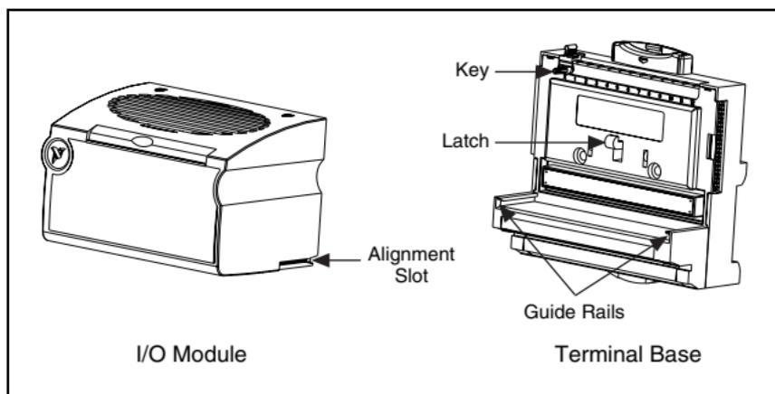
Figure 1. Installing the FP-AI-102
