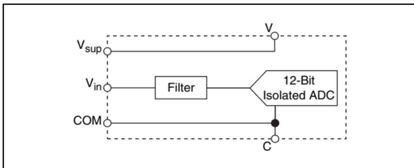
**Figure 3.** [c]FP-AI-102 Analog Input Circuit, One Channel
