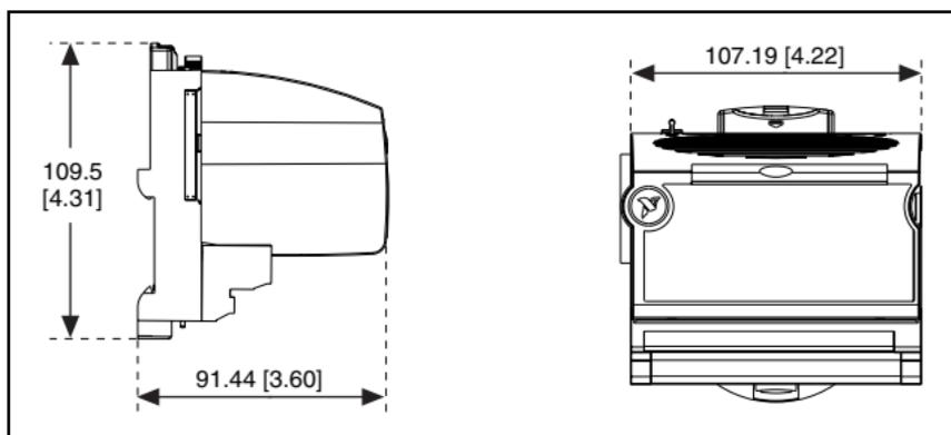
**Figure 6.** FP-AI-102 Mechanical Dimensions
