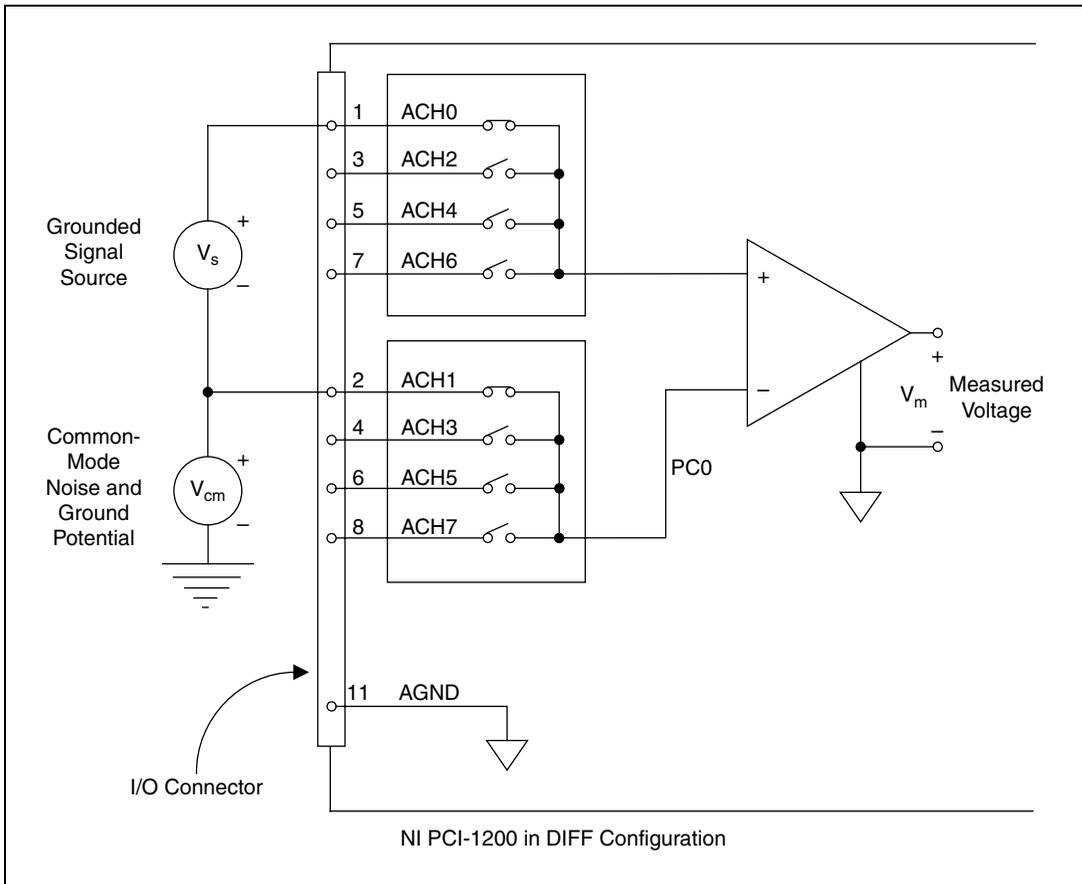
**Figure 3-3.** Differential Input Connections for Grounded Signal Sources
