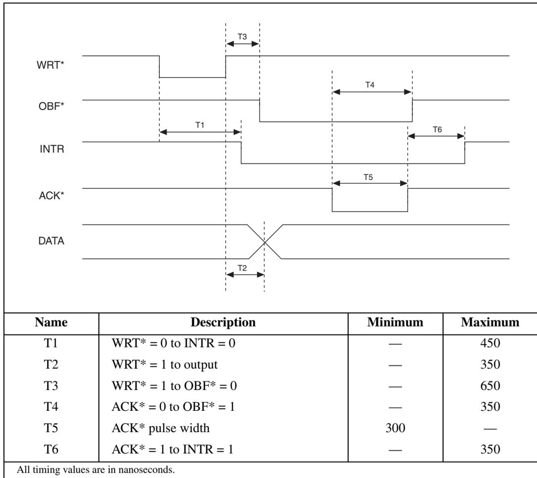
**Figure 3-18.** Mode 1 Timing Specifications for Output Transfers
