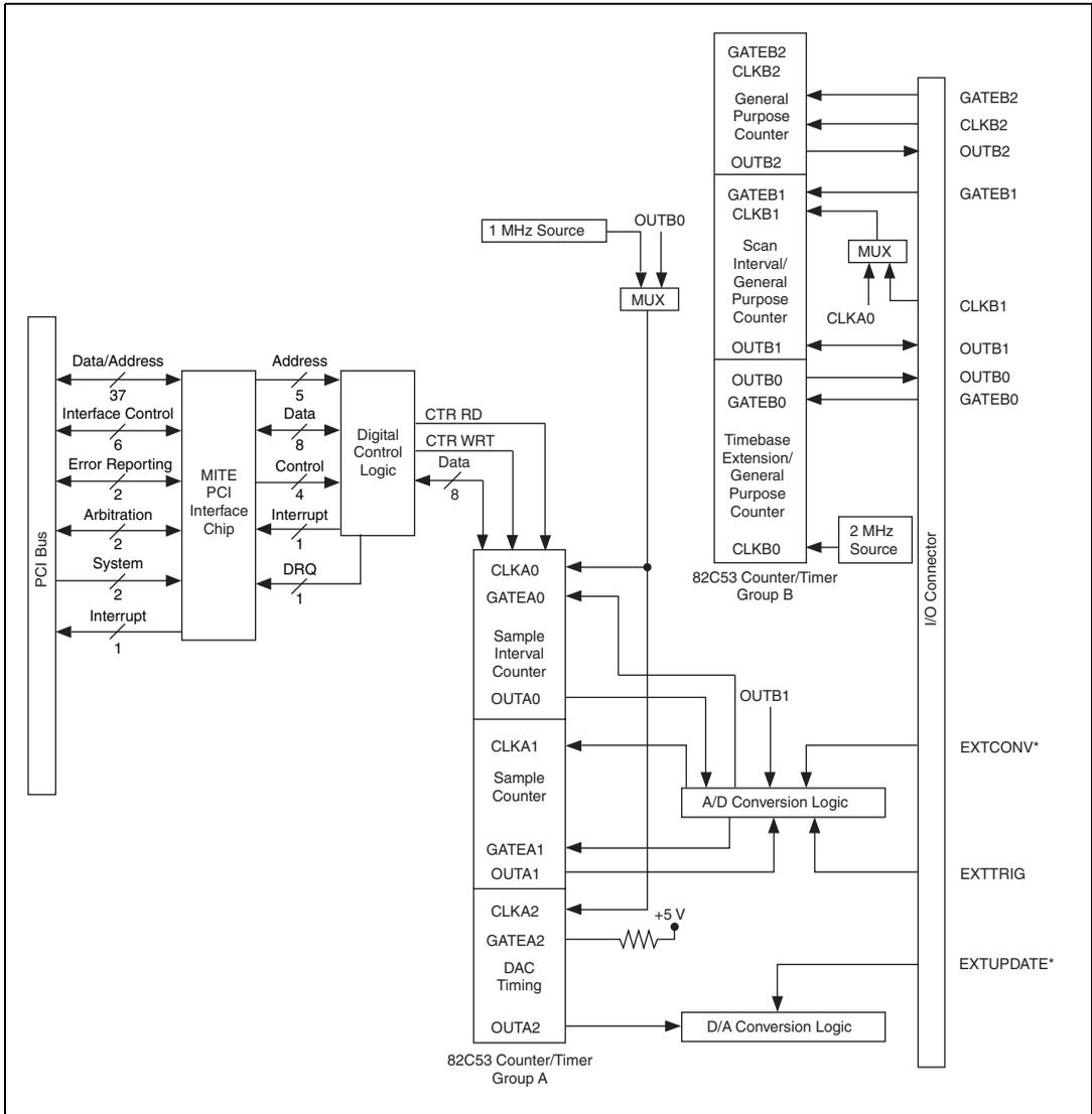
**Figure 4-3.** Timing Circuitry
