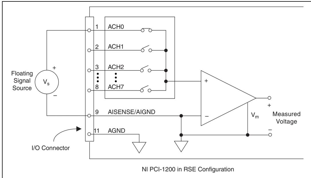
**Figure 3-5.** Single-Ended Input Connections for Floating Signal Sources
