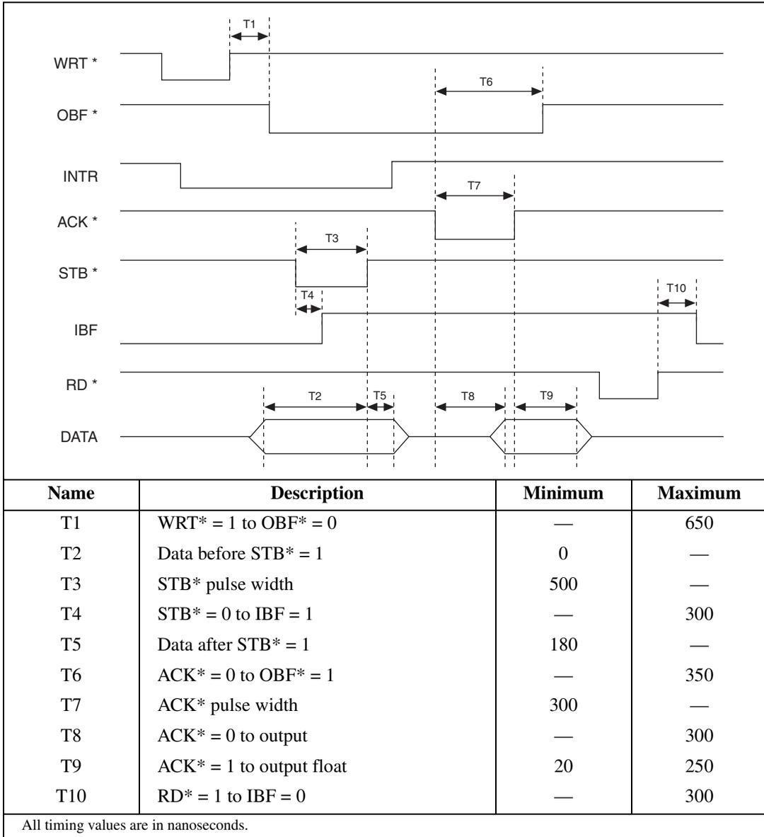
Figure 3-19. Mode 2 Timing Specifications for Bidirectional Transfers
