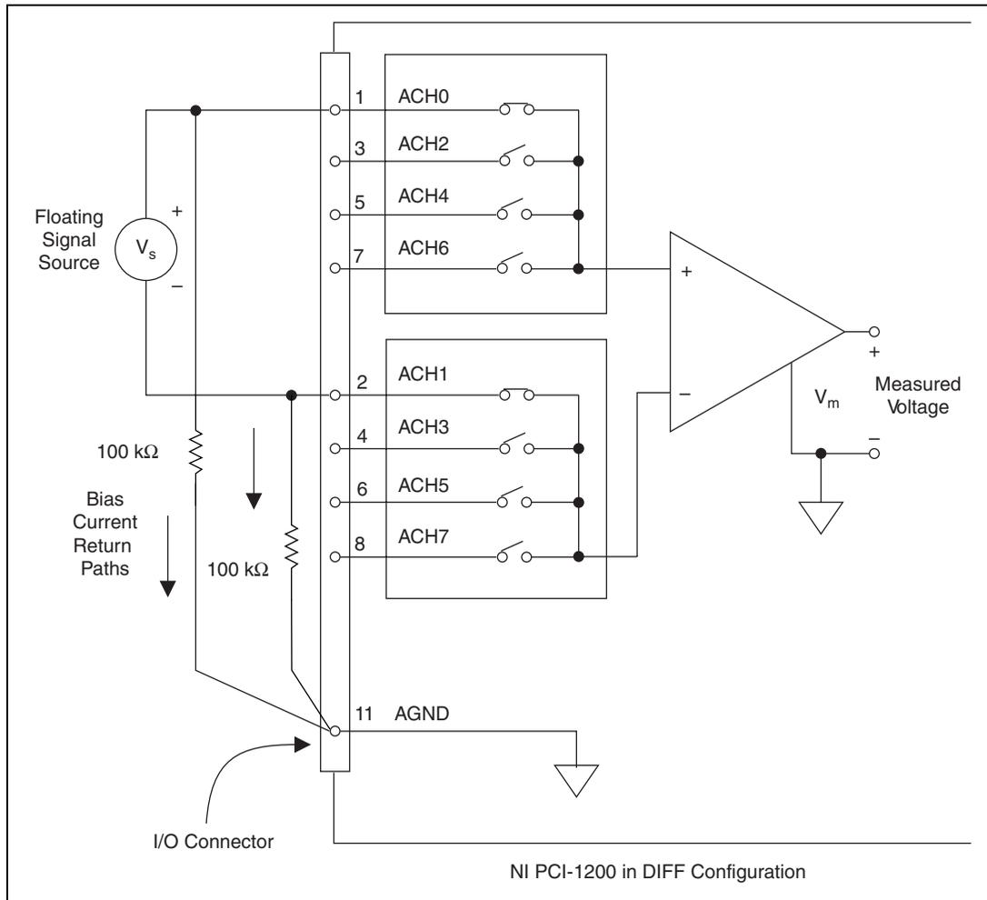
**Figure 3-4.** Differential Input Connections for Floating Sources
