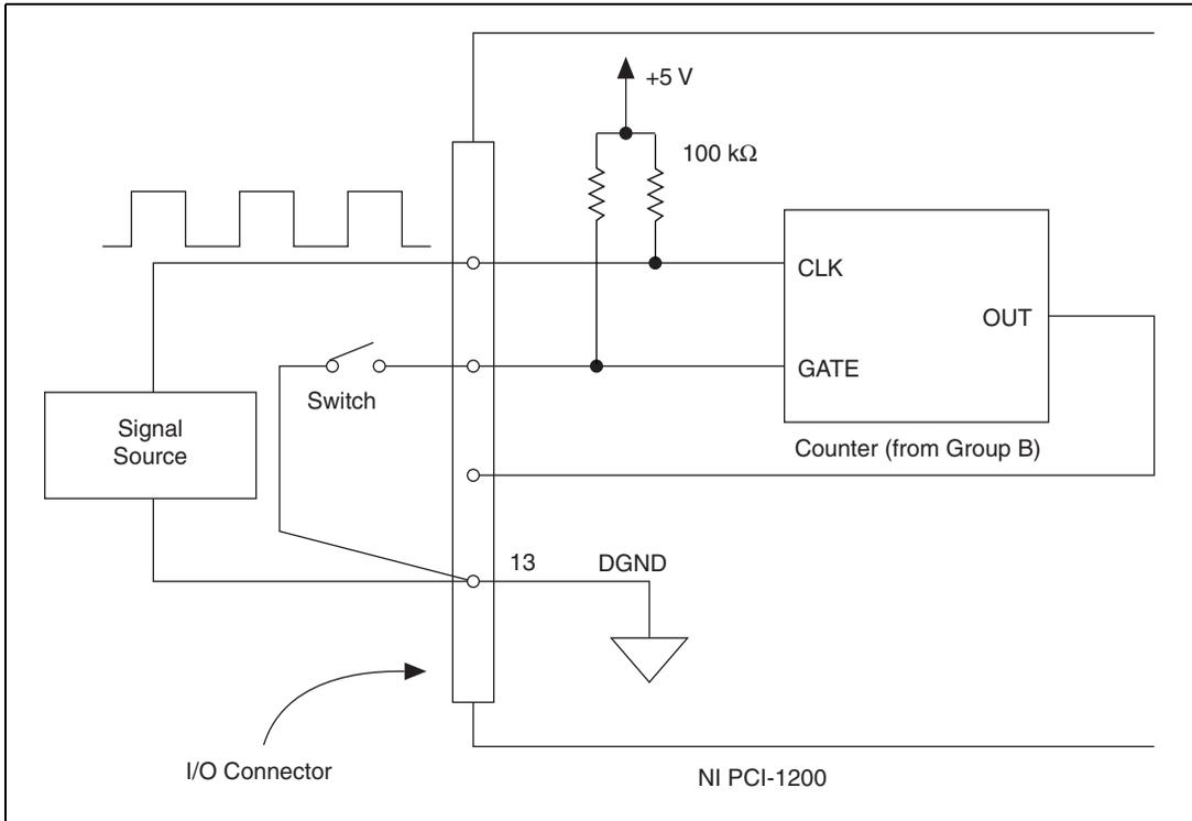
**Figure 3-14.** Event-Counting Application with External Switch Gating
