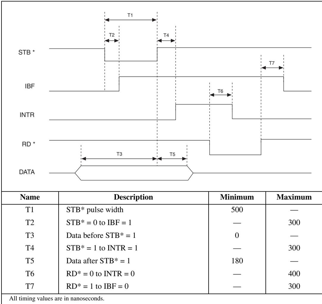
**Figure 3-17.** Mode 1 Timing Specifications for Input Transfers
