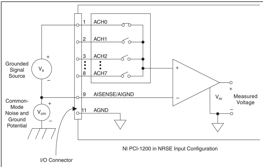
**Figure 3-6.** Single-Ended Input Connections for Grounded Signal Sources
