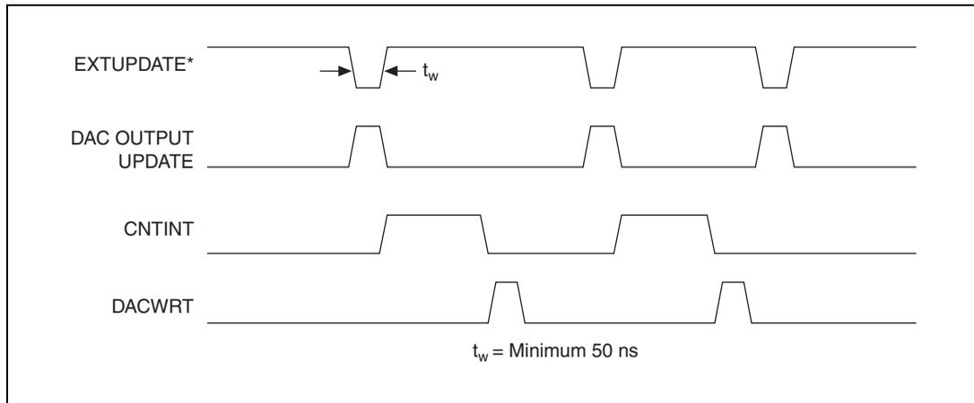
**Figure 3-13.** EXTUPDATE\* Signal Timing for Updating DAC Output
