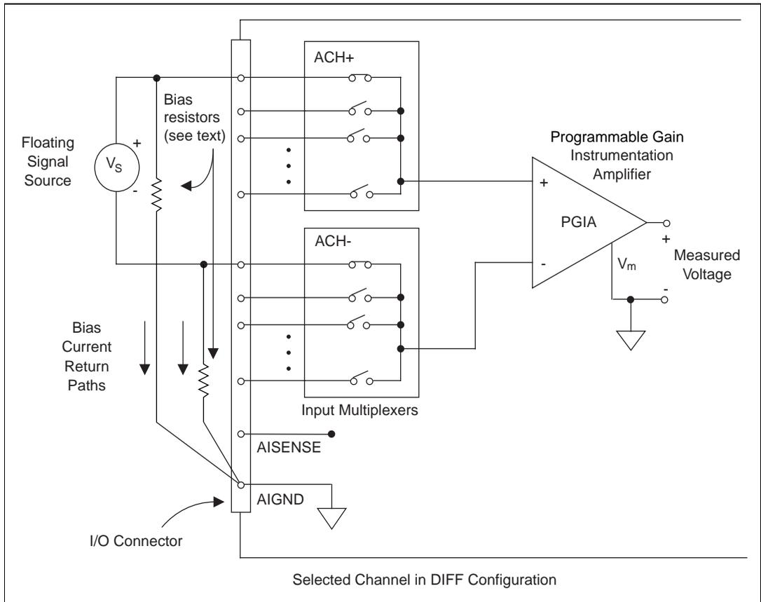
**Figure 4-6.** Differential Input Connections for Nonreferenced Signals
