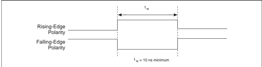
**Figure 4-39.** GPCTR1\_GATE Signal Timing in Edge-Detection Mode
