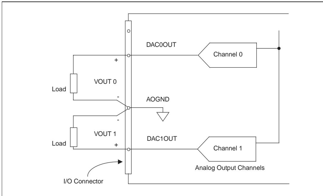
**Figure 4-9.** Analog Output Connections
