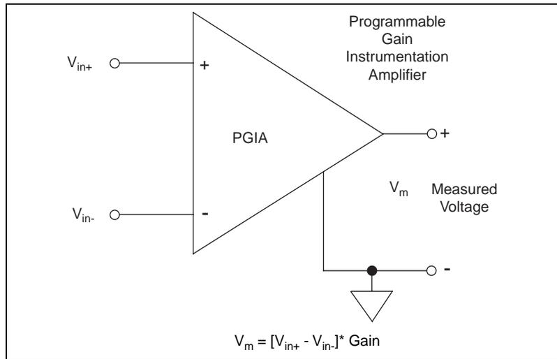
**Figure 4-3.** Programmable Gain Instrumentation Amplifier (PGIA)
