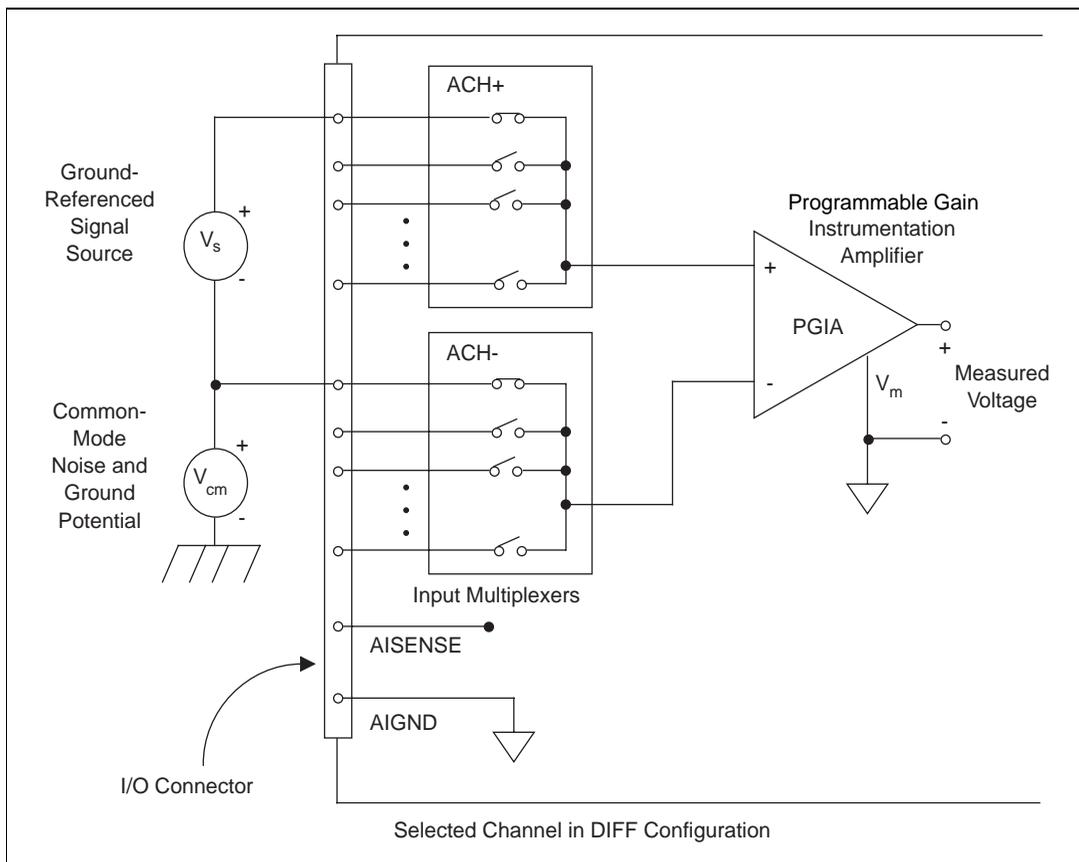
**Figure 4-5.** Differential Input Connections for Ground-Referenced Signals
