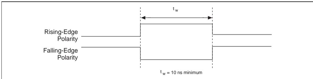
**Figure 4-36.** GPCTRO\_GATE Signal Timing in Edge-Detection Mode
