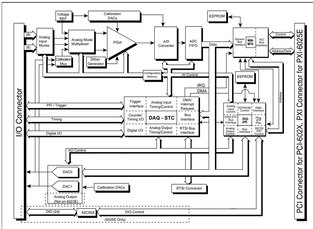
**Figure 3-1.** 6023E, 6024E, and 6025E Block Diagram
