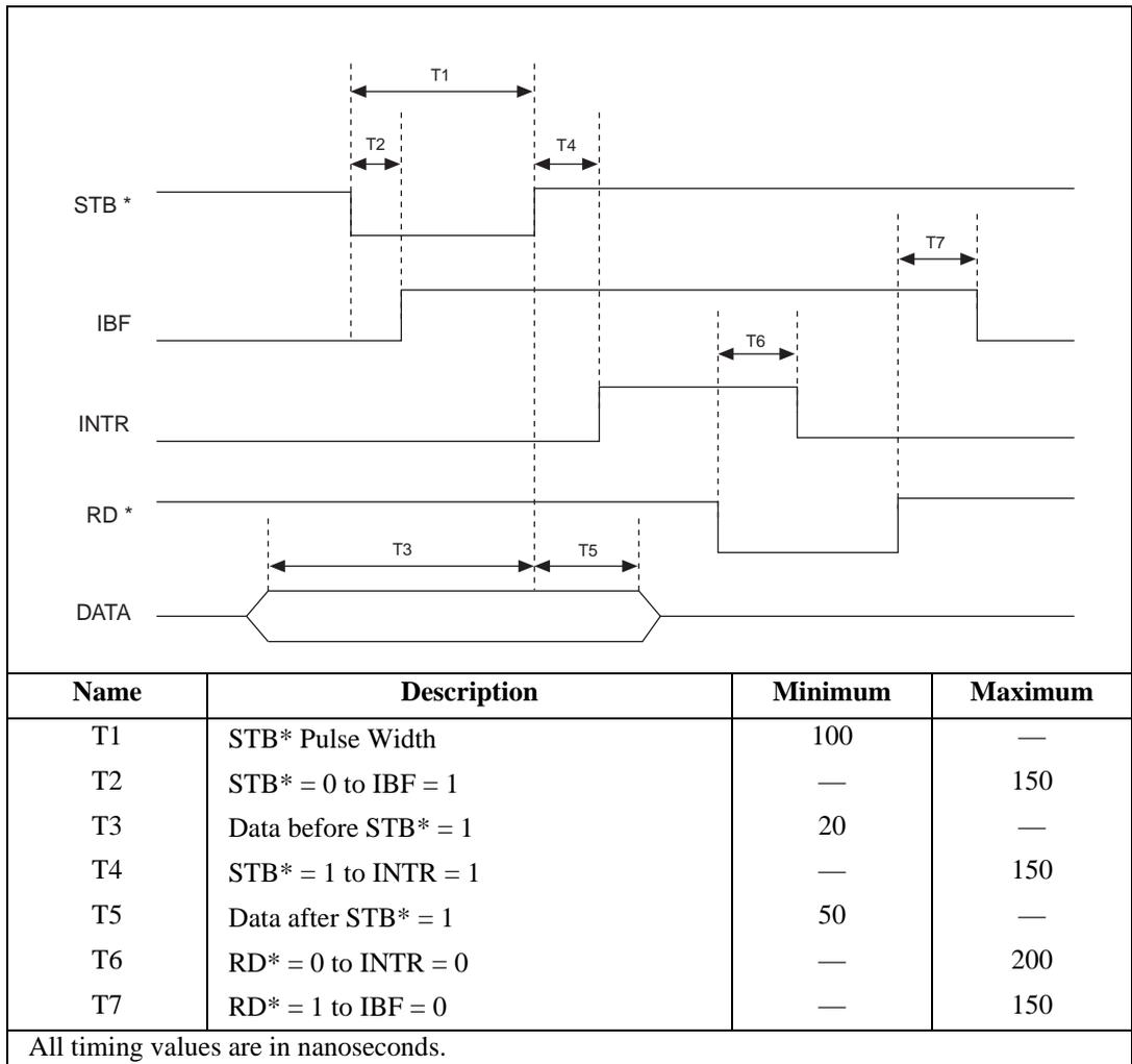
**Figure 4-13.** Timing Specifications for Mode 1 Input Transfer
