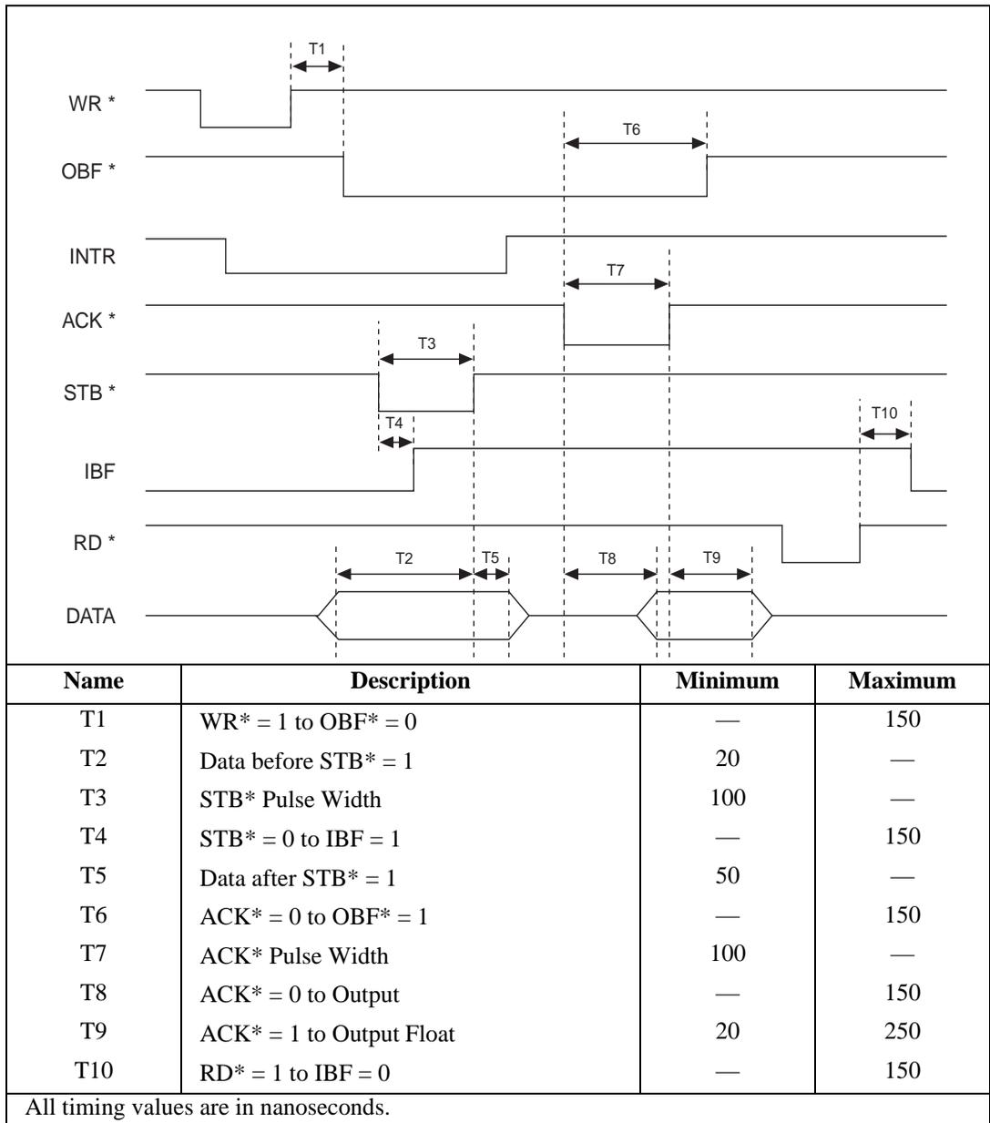
**Figure 4-15.** Timing Specifications for Mode 2 Bidirectional Transfer
