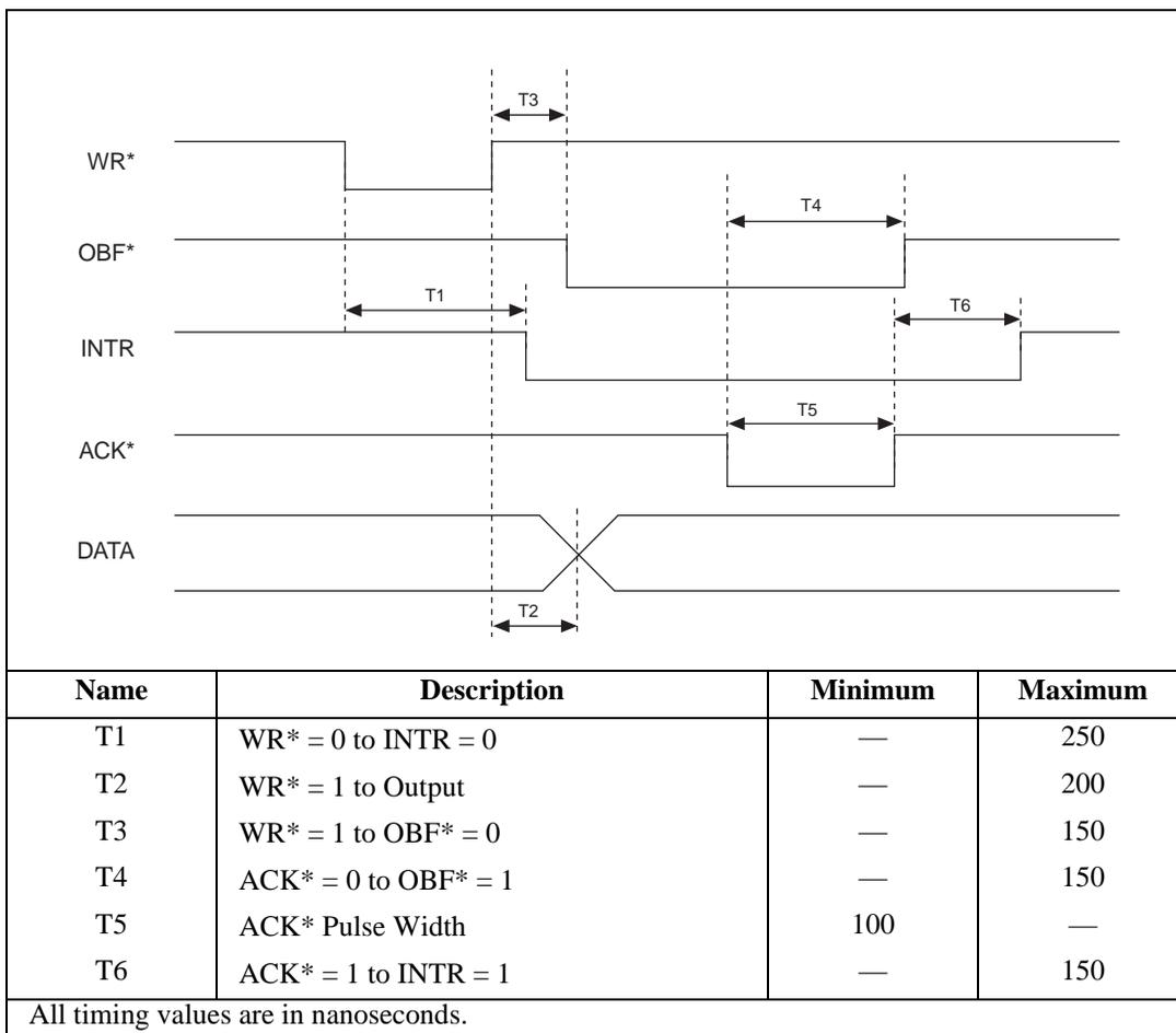
**Figure 4-14.** Timing Specifications for Mode 1 Output Transfer
