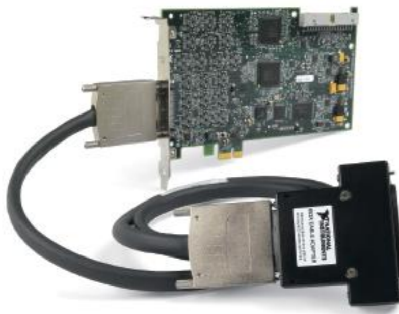
Figure 2. You can use NI 6535/36/37 devices with an NI 653x cable adapter to connect to existing NI 6533/34 applications.
