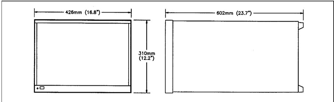
Mainframe weight ..... 22 Kg (48.5 lbs) with no modules installed
