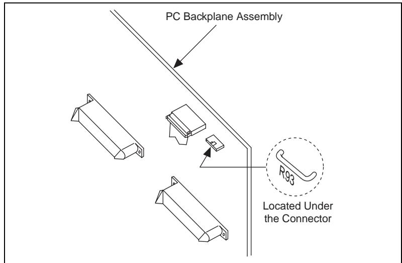
**Figure 1-4.** Location of R93 Surface Mount Resistor
