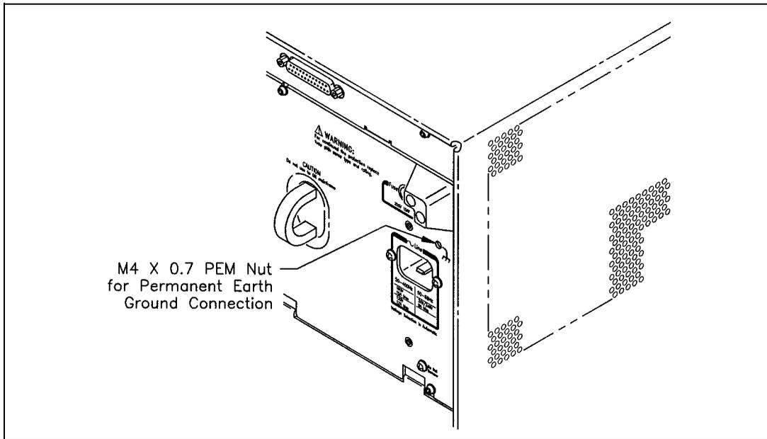
Figure 1-6. Grounding Connection
