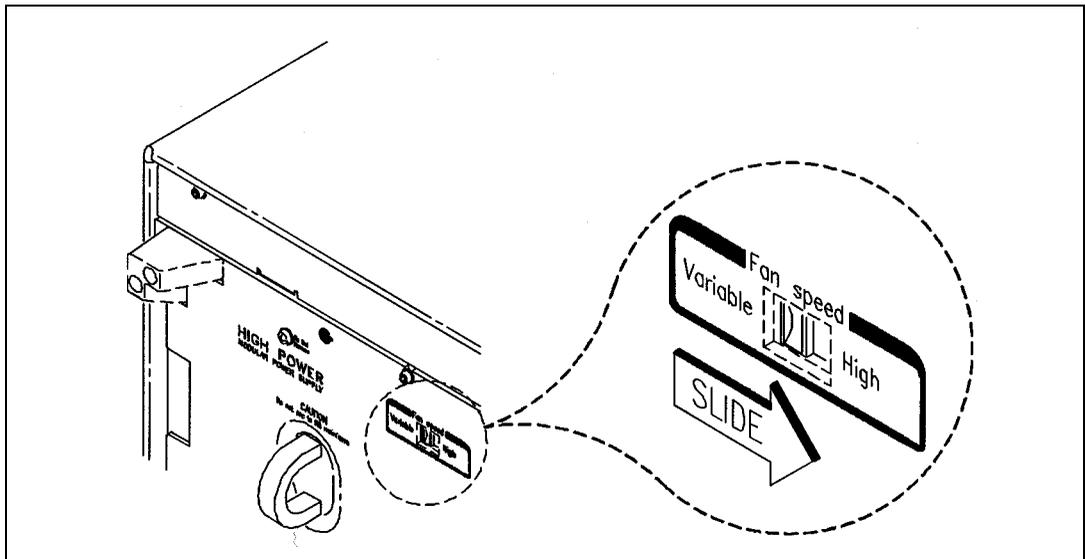
Figure 1-2. Forcing the Fan to High Speed
