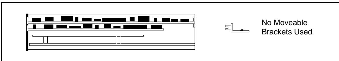
Figure E-15. First Board between 8.2 in. and 13.4 in. Long, Second Board Full 13.4 in. Long
