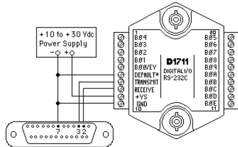
Note: If using a DB-9 connector ground is tied to pin 5 only. Pin 2 is tied to TRANSMIT and pin 3 is tied to RECEIVE on the module.
