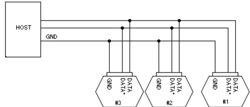
It is possible to configure two or more modules to Continuous Output Change mode on the same serial port.
