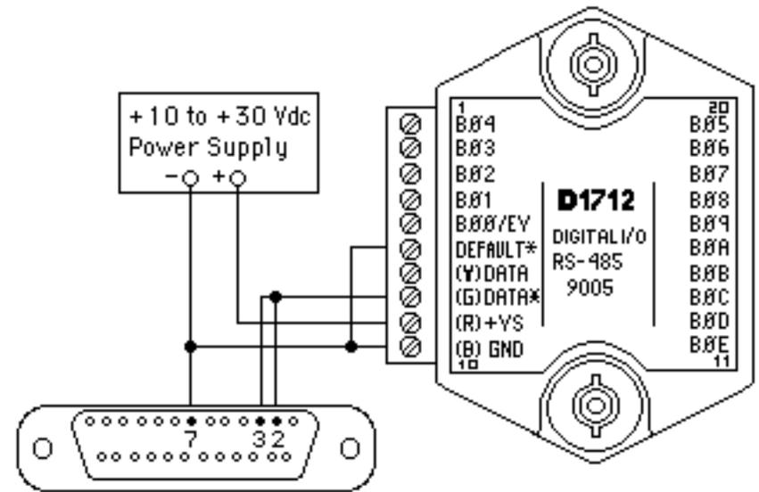
Note: If using a DB-9 connector ground is tied to pin 5 only.
