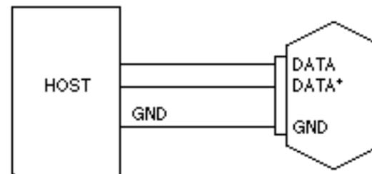
A D1712 module set up for change mode will output a data string if one of its digital input lines has changed state. The module will output the data string reporting the new state of the inputs.
