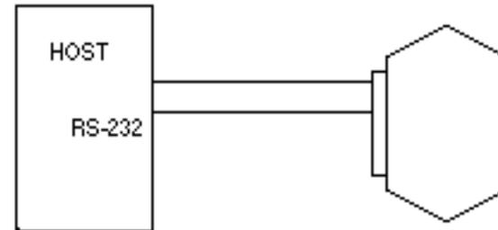
In this configuration, a D1712 module is set to continuously output data to a host computer or display device. It is not necessary for the host to poll the D1712 to obtain data. The host computer must have an interrupt-driven serial input for proper operation.
