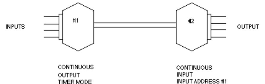
Module #1 is setup in Continuous Output Timer Mode as described in Example A. Module #1 will read the state of the digital inputs and produce data messages on the communications bus. In this application, setting the Continuous Timer to zero will produce the fastest response to input changes.
