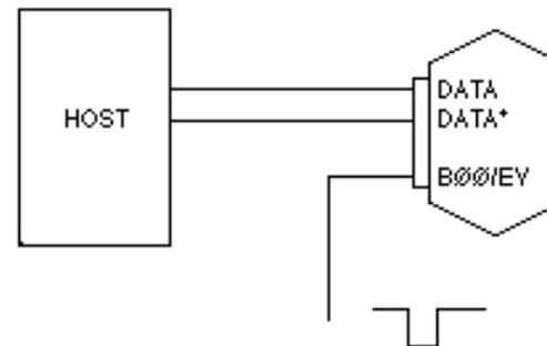
The external trigger signal is connected to the B00/EV pin of the module. Since the B00 pin is used for the trigger, it is not available for general-
