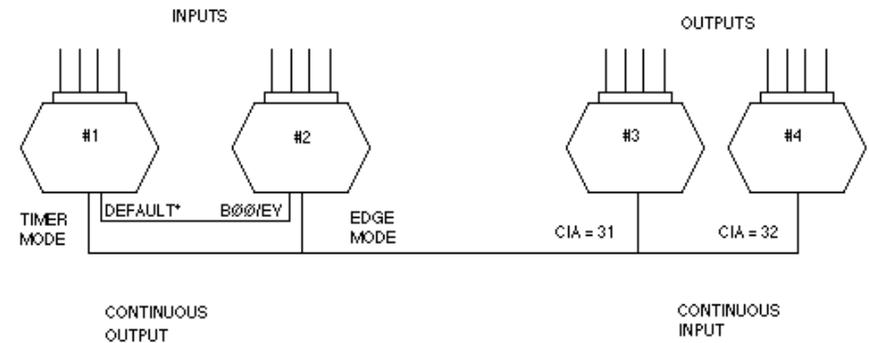
This system is similar to example E except that 2 input-output module pairs share the same communications line. Modules #1 and #2 are setup for continuous output as detailed in example B. This pair of D1712's constantly read the state of their respective digital I/O lines and output the data on the communications bus. A typical output data stream would be:
