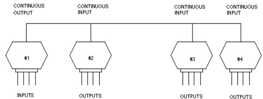
In this system, module #1 is set for Continuous Output mode. Modules 2, 3 & 4 are setup for Continuous Input. The three Continuous Input modules are all setup with a Continuous Input Address (CIA) of ASCII 31 or character '1'. This means that each of these three modules will accept the data from module #1 as an output command. The outputs of modules 2, 3 and 4 will replicate the input data of module #1.
