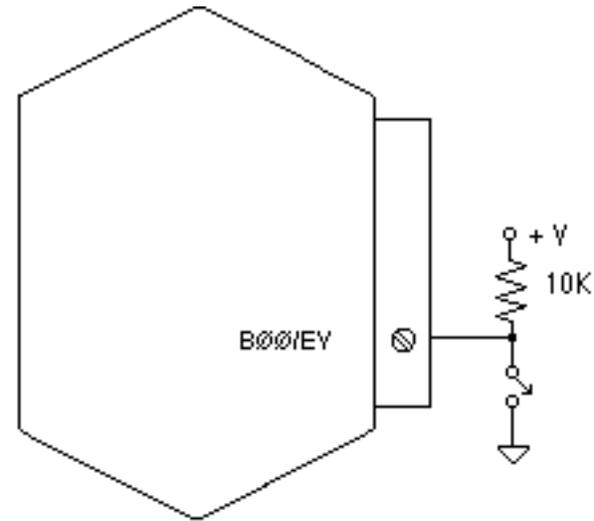
The module is triggered on a positive-going edge to the B00/EV pin. To setup the D1712 for edge-trigger mode:
