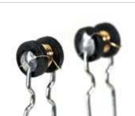
▼ Solder point inspection of copper wire.
