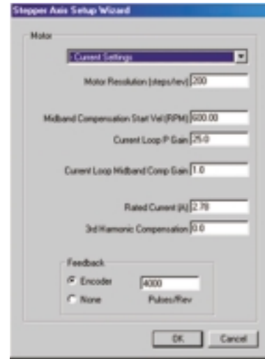
ToolPAC's Setup Wizard makes drive configuration easy.
