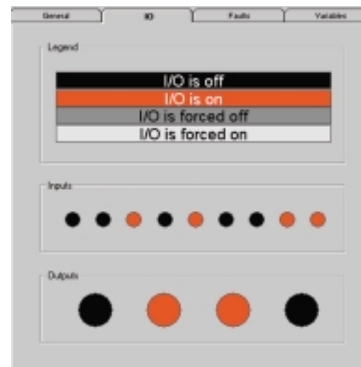
ToolPAC gives you status and full control of I/O points for programming and trouble shooting.
