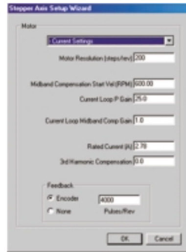
ToolPAC's Setup Wizard makes drive configuration easy.
