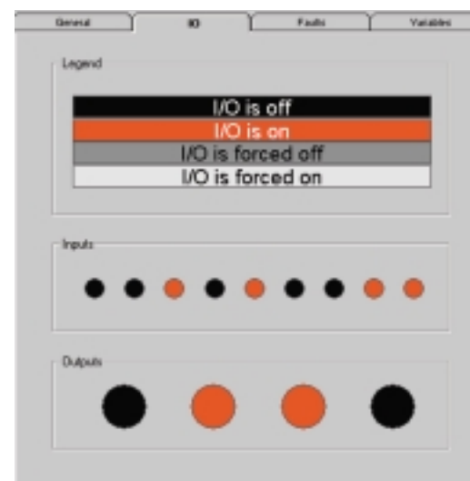
ToolPAC gives you status and full control of I/O points for programming and trouble shooting.
