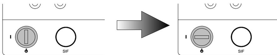
The main 'Power On' switch is a key switch located on the front panel. Insert the key and rotate clockwise 90 degrees to switch the unit on. The key can only be inserted or removed when it is in the vertical 'Off' position. The unit will perform a short initialization and check procedure lasting about one minute. The display will sequence through the following patterns.
