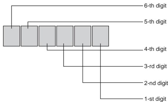
The SU command is provided to enable the current status of the rotating polarizer and the measurement speed setting to be probed. The command returns a six digit number. The interpretation of the six digit number is detailed overleaf:
