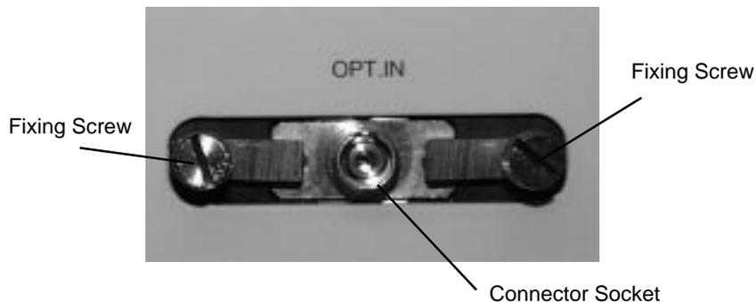
1. Unscrew the two fixing screws on either side of the optical connector socket.
