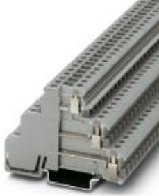
Sensor/actuator terminal block, Cross section: 0.2 mm 2 - 4 mm 2 , AWG: 24 - 12, Connection type: Screw connection, Width: 6.2 mm, Color: gray, Mounting type: NS 35/7.5, NS 35/15
