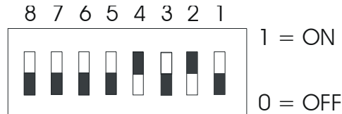
Fig. 3: DIP-Switch Settings (switch slider shown in black)
