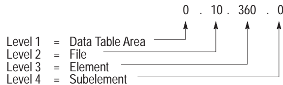
Figure 6.8 PLC-5 Logical Binary Addressing
