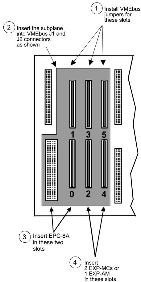
The EXP-BP4A subplane is used in systems needing a CPU and six EXM modules.
