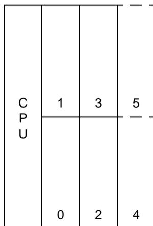
Figure 3-10. Slot Numbering
