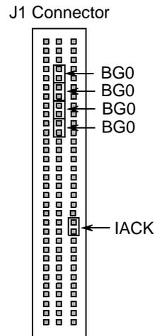
**Figure 2-4. VMEbus Jumpers on Rear Wirewrap Pins**
