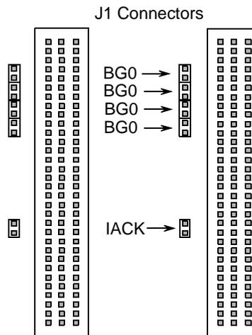
**Figure 2-5. VMEbus Jumpers on Front Stake Pins**
