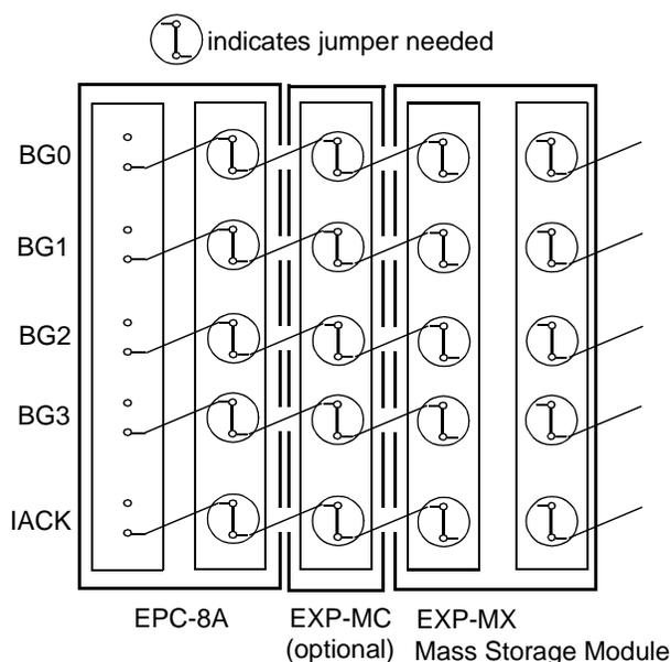
**Figure 2-3. Backplane Jumpers Required for EPC-8A Subsystem**
