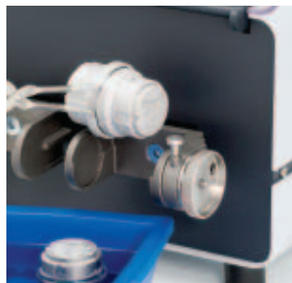
Before grinding takes place the grinding jars are immersed in liquid nitrogen (-196 °C) in the cryo box for approx. 2 - 3 minutes
