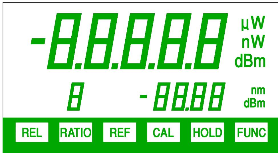
Figure 4-1 LCD segments and annunciators.
