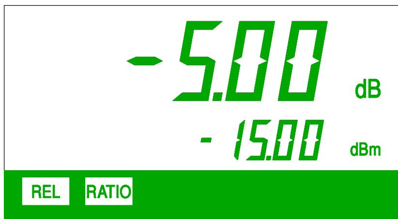
Figure 4-4 LCD display while in REL+RATIO mode.
