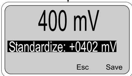
5. The number on the large display is the live process ORP reading. The next line displays the ORP reading when the display was accessed. Press Edit (F4) to perform the standardize.
