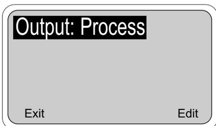
To make changes in these parameters, highlight the desired menu header and press Enter [F4]. The value now being used is displayed and the F4 key can be pressed to Edit the item. Once Edit has been pressed, change the item as needed and then press Save [F4] to store the value. Repeat for the other output and/or items as needed.
