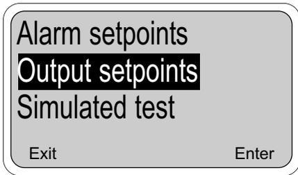
This section describes how the 4 (or 0) to 20 mA current outputs can be reranged. Note that the current outputs can be configured to represent pH, temperature, glass impedance, or reference impedance. See Section 5.6 for details on configuration.
