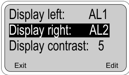
4. This screen allows you to choose the items displayed on the third line left and right of the main display screen. The process temperature and output 1 value (in mA or %) are always shown on line 2 of the main display. This screen allows you to make the following choices:
