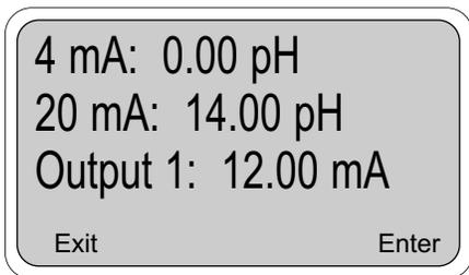
This screen allows changing the setpoints for output 1. A similar screen is available for output 2. The live current output now being transmitted by the controller is shown on the third line.
