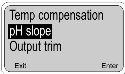
The slope of the glass electrode is normally calculated during buffer calibration. It can, however, be entered directly (if known) using this procedure. A new electrode has a slope of about 59 mV/pH but as it ages the slope will decrease. A slope value below 47 mV/pH unit is a sign of an aged electrode and is not considered adequate for calibration. The pH slope can also be viewed on the diagnostic variables screen.
