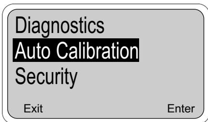
This section describes how the controller may be set up for auto calibration, which includes automatic buffer recognition and auto stabilization. Alternatively, the controller may be configured to perform a manual calibration without the automatic features.
