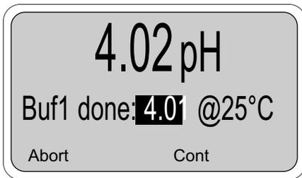
3. A screen like the one on the left will appear after stabilization.
