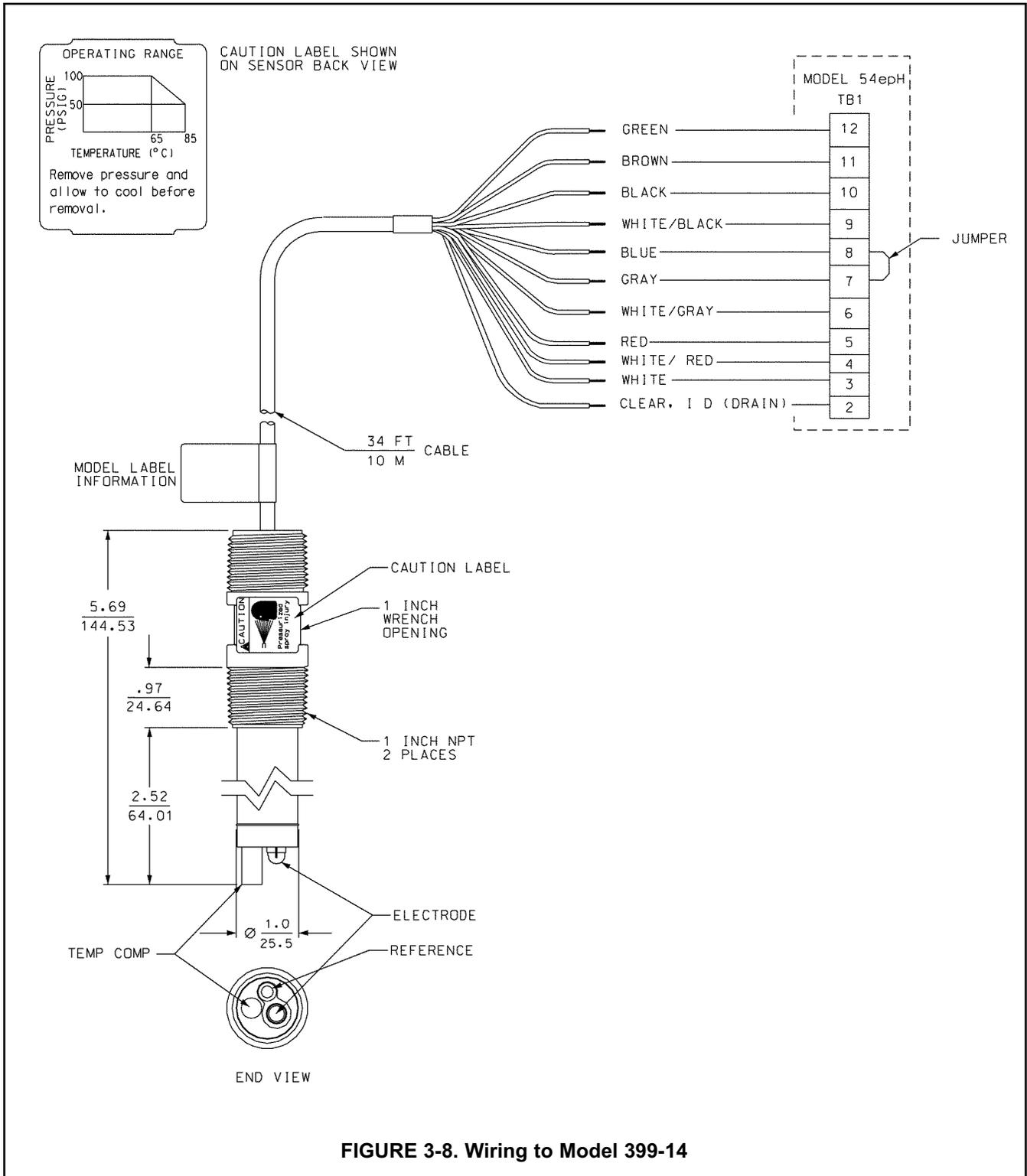
FIGURE 3-8. Wiring to Model 399-14
