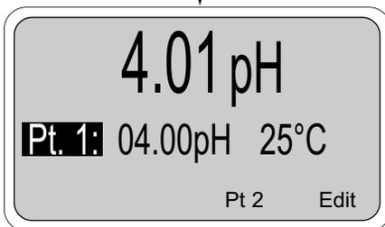
4. Press Pt 2 (F3) to enter Buffer 1 into memory and proceed to buffer 2 (pt. 2) calibration.
