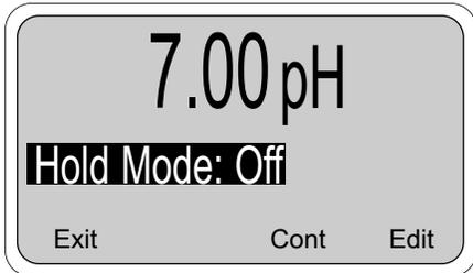
The two-point calibration is performed when the controller is initially installed and whenever elements of the sensor assembly or controller are replaced. The two-point calibration re-establishes the slope of the electrode. This is necessary because the slope (mV/pH change) decreases as the glass pH electrode ages.
