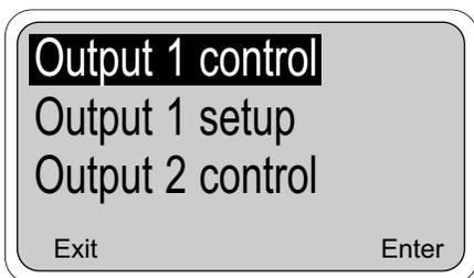
2. There are 5 menu headers that relate to outputs. Each output has a control header and a setup header. In addition, the hold feature is turned on here. The hold feature is mostly used to prevent upsets during buffer calibration of the pH sensor.
