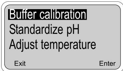
1. From the main display, press any key to obtain the main menu. With the cursor on "Calibrate", press Enter (F4). With the cursor on "Buffer calibration", press Enter (F4) again.
