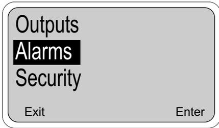
This section describes the options available for configuration of the alarms. Alarms 1, 2, and 3 can be activated on pH (or ORP/Redox, see Appendix A), or temperature. One of these alarms can be setup as a feed limit timer and another alarm can be dedicated as an interval timer. Alarm 4 is reserved as a fault alarm.
