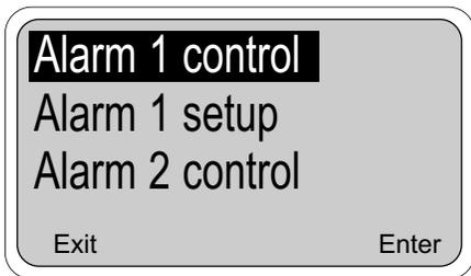
2. There are 9 menu headers that relate to alarms. Alarms 1, 2, and 3 each have a control header and a setup header. Alarm 4 has a simple setup header. Configuration of a feed limit timer and an interval timer is also described here.
