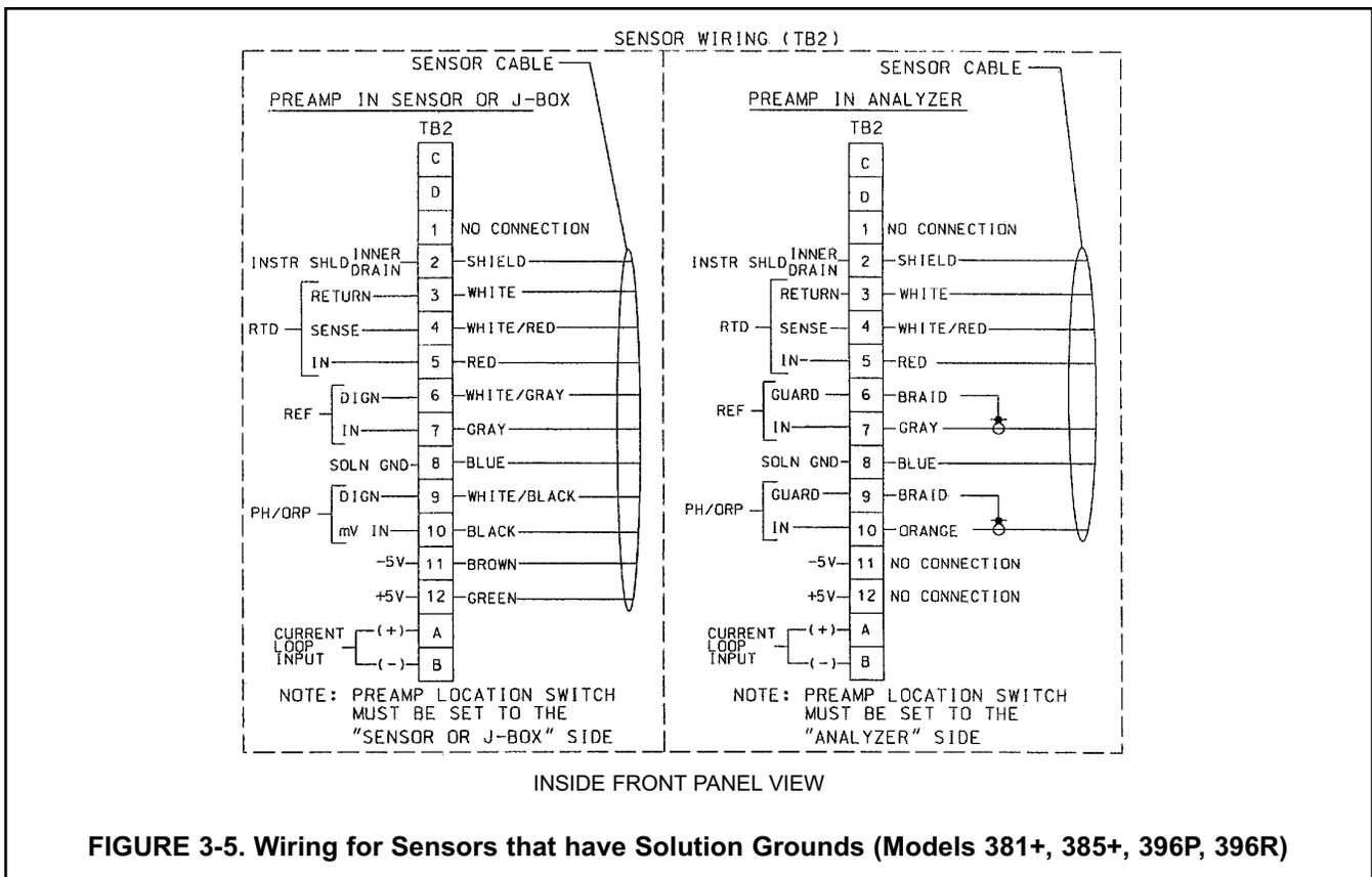
FIGURE 3-5. Wiring for Sensors that have Solution Grounds (Models 381+, 385+, 396P, 396R)
