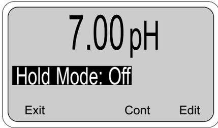
Placing the Controller on Hold for Maintenance. Before performing maintenance or repair of the sensor, the Controller can be placed in hold (refer to Section 5.6 to enable this feature) to prevent process upsets while the reading is off-line. This will place the current outputs into the selected default states (see Section 5.6). The relays will act as selected in relay default, see Section 5.7.
