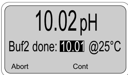
5. A screen like the one on the left will appear after stabilization. **Use the arrow keys to select the correct buffer, and press Cont (F3).** If the correct buffer does not appear, refer to Section 5.9 and select a buffer group that includes the desired buffers. As usual, to cancel the calibration, press Abort (F1).
