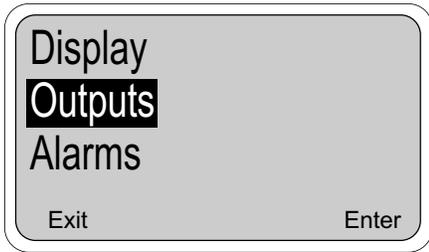
This section describes the options available for configuration of the outputs. Each output can be configured to represent pH (or ORP/Redox, see Appendix A), temperature, glass impedance, or reference impedance. In addition, each output can be linear (normal) or nonlinear (PID). Several options for both modes of outputs can be configured. This section describes the features and shows how to make modifications in the settings.
