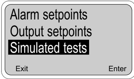
This section describes how the current outputs and alarm relays can be manually set for the purposes of checking devices such as valves, pumps, or recorders.
