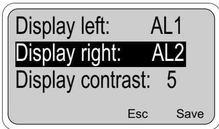
The "Display contrast" selection allows the display to be made lighter or darker. Entry 0 is the lightest and 9 is the darkest. The display changes as the number is changed.
