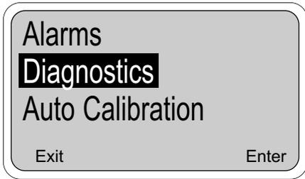
This section describes the options available for configuration of the on-line sensor diagnostics. The controller checks the integrity of the glass electrode (for pH only) and the reference electrode by continuously measuring the impedance of each. The original controller configuration is with diagnostic messages turned off. To enable this feature, see below.
