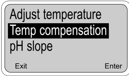
Automatic Temperature Compensation is a standard option for pH equipment and is used in virtually all pH measurement situations. If compensation is not desired, the temperature signal from the sensor can be ignored by placing the controller in the manual temperature compensation mode.
