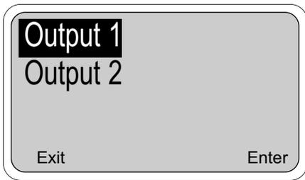
2. Select the desired output by moving the cursor down to highlight it. When the correct output is highlighted, press Enter (F4) to get to the adjustment screen.
