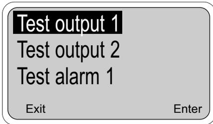
2. At this point there are six separate screens for testing each of the current outputs and each of the alarm relays. Highlight the desired item by pressing the arrow **[↓]** **[↑]** keys as needed.
