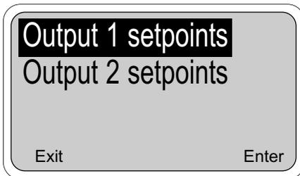
2. Highlight the desired Output setpoints and press Enter (F4).
