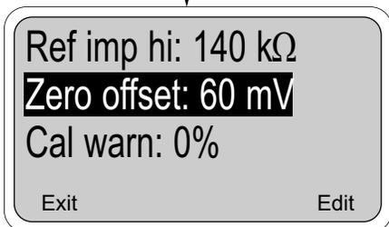
The values now being used by the controller are displayed. To change any of these items, use the arrow key to highlight the desired item and press Edit(F4). Use the arrow keys to make the change and press Save(F4) to enter the change into memory.
