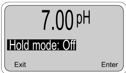
When the hold feature has been enabled, this Hold Mode Screen will appear when the Calibrate routine is entered. Possible actions are Exit **[F1]** which cancels the calibration, Enter **[F4]** which enters the calibrate menu without putting the controller in hold, and Edit **[F4]** which allows turning Hold Mode On. Note that when hold has been enabled, this screen requires pushing Cont **[F3]** to enter and leave the calibrate menu.
