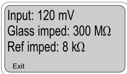
3. Diagnostic variables are displayed three at a time. More variables are viewable until the cursor (showing highlighted text) is brought down to the bottom line.
