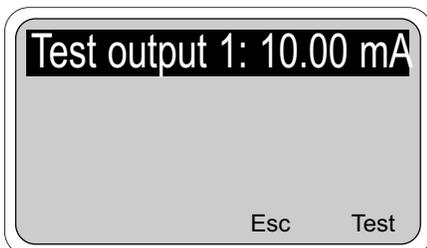
If the displayed current is not the desired value, press the Edit **[F4]** key and the next screen will allow changing the value. Use the arrow keys to change the display as needed, and press Test **[F4]** to use that value. Press Esc **[F3]** to cancel the change in the value and continue simulating the previous current.
