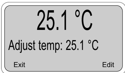
3. Press Edit (F4) with this display shown to adjust the temperature. The screen below will then appear. Using the arrow keys, input the correct temperature value and press Save (F4). The controller will enter the value into memory. To abort the change, press Esc (F3). Afterwards, to continue with buffer calibration, go to Section 4.2 or 4.3, otherwise press Exit (F1) three times for the main display.
