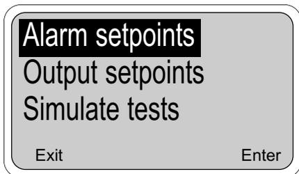
This section describes how the three alarm setpoints can be changed. Move the cursor down by pressing the arrow key.
