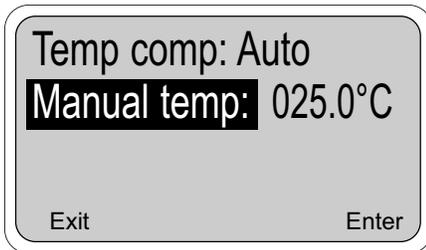
To change these settings, obtain the top screen by pressing Enter (F4) when Calibrate is highlighted in the main menu and then press the arrow key. Press Enter (F4) again to obtain the lower screen. Highlight the desired item and press Edit (F4) and change the value as needed. Options are Auto or Manual temperature compensation and the temperature values listed above. Press Save (F4) to save the change. Esc (F3) will cancel the change.
