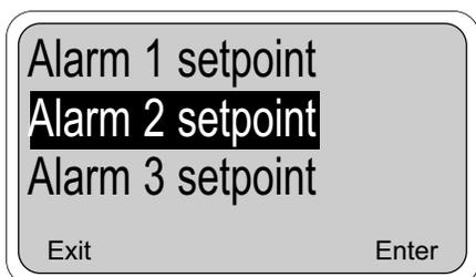
2. Select the desired alarm by moving the cursor down to highlight it. When the correct alarm is highlighted, press Enter (F4) to get to the adjustment screen.
