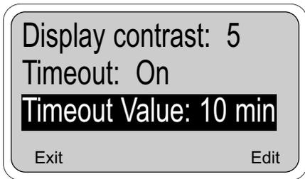
5. The timeout feature works on both the display and simulated tests using the current outputs and alarm relays.
