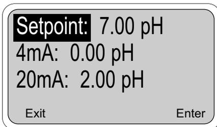
3. The setpoint now being used is displayed. Press Edit (F4) and use the arrow keys to change the display to the new value.
