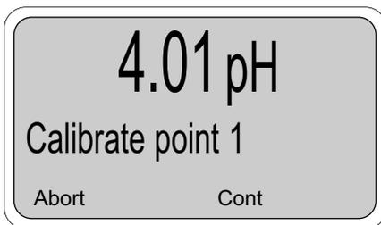
2. Place the sensing portion of the pH sensor into a beaker containing the first buffer solution. The large displayed pH shows the actual pH.
