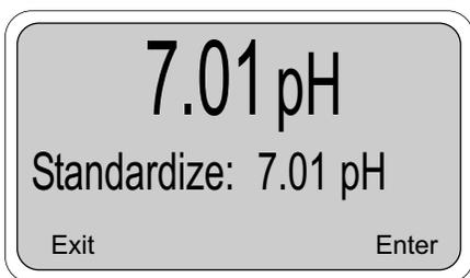
5. The pH reading in large numbers is the live process pH reading. The next line displays the pH reading when this screen was first accessed. Press Edit (F4) to perform the standardize.
