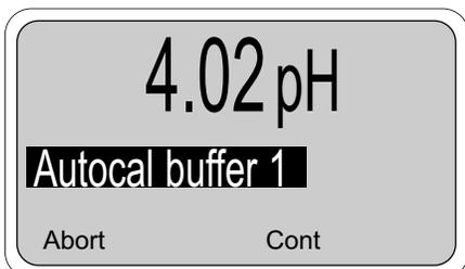
2. With the sensor in the first buffer, press Cont (F3). To cancel the calibration, press Abort (F1.)
